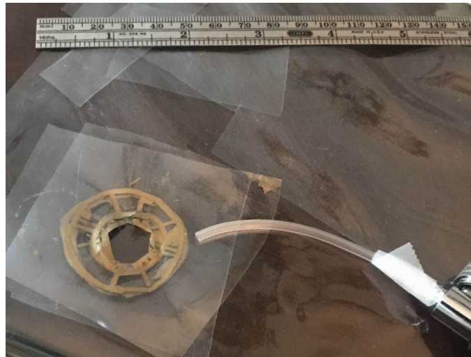
Figure 17: The first prototype of the balloon was constructed by measuring and cutting vinyl sheets.
