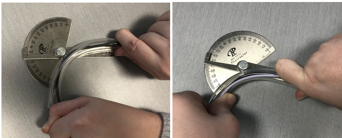
Figure 21: Picture of measuring angle of catheter without swab (left) and with swab (right)
