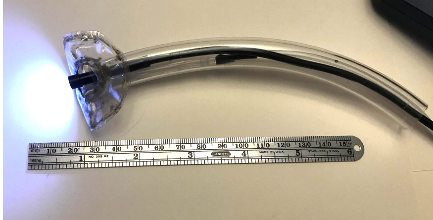
Figure 18: The first version of the prototype, with the camera and light at the cervix-end of the device connected to the monitor. The balloon is also at the cervix end and is fed through an air tube.
