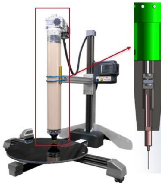
Figure 27 Schematic of the ceramic robocasting machine with a customized extruding unit [76].
