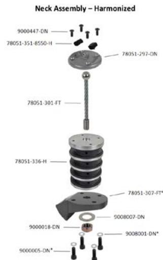
Figure 15: Hybrid 3 Test Dummy Neck
