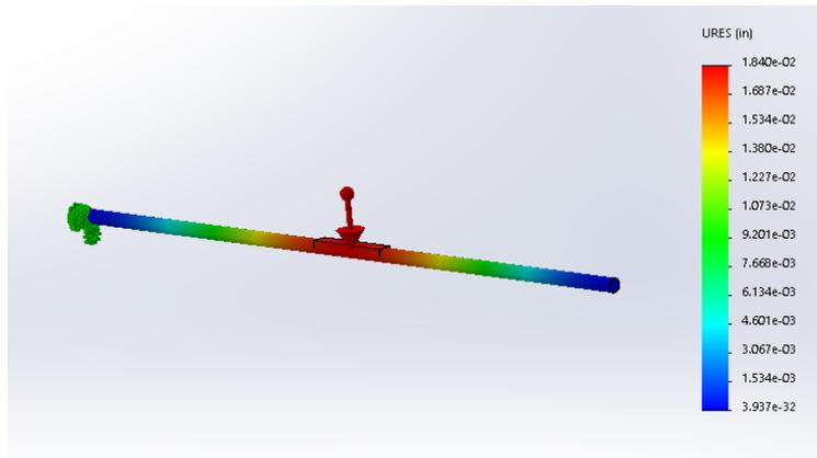
Figure 28: SolidWorks Testing of the Horizontal Beam
