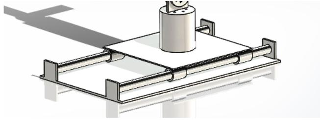
*Figure 25: Linear Sliding Rails of the Test Dummy*
