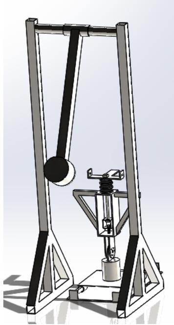
*Figure 23: Pendulum Testing Rig*
