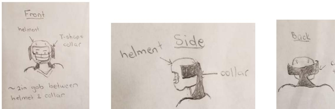
Figure 32: T-Bracket Design Multi View
