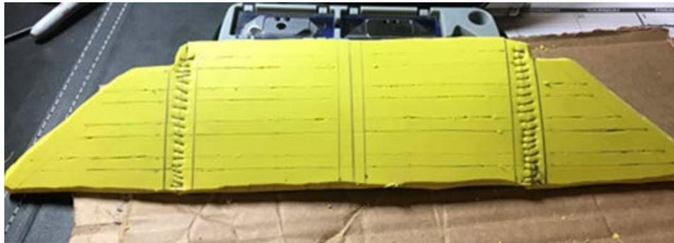
*Figure 38: Final 3-piece Foam design sewn together*
