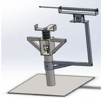
Figure 22: Pneumatic Cylinder Test Rig
