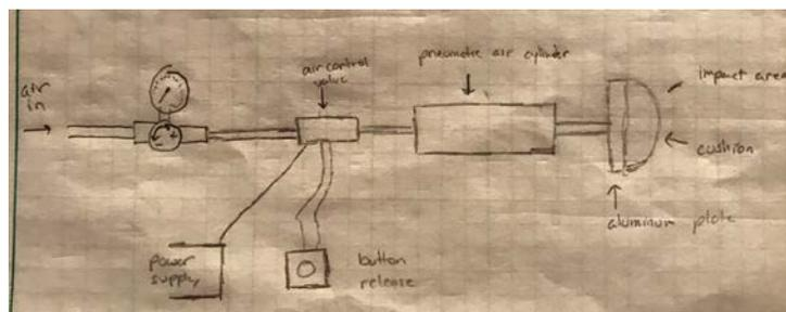
Figure 21: Hand Sketch of Compressor to Cylinder
