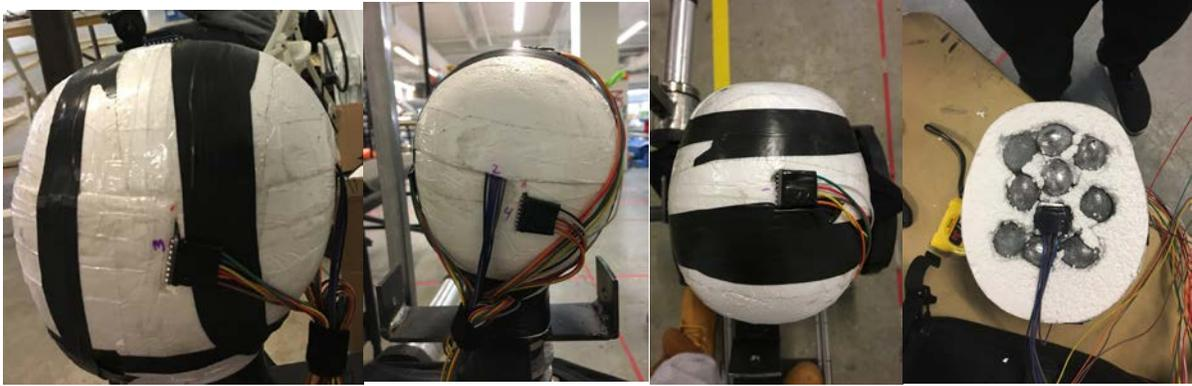
*Figures 41: 4 Accelerometers placed in weighted Styrofoam head*
