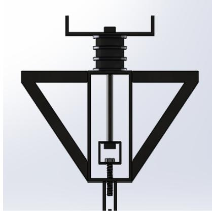
*Figure 17: SolidWorks Design of Tensioning Device*
