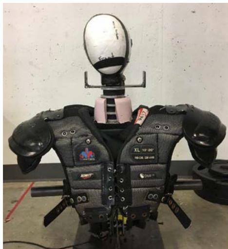
*Figure 19: Test Dummy with Shoulder Pads*
