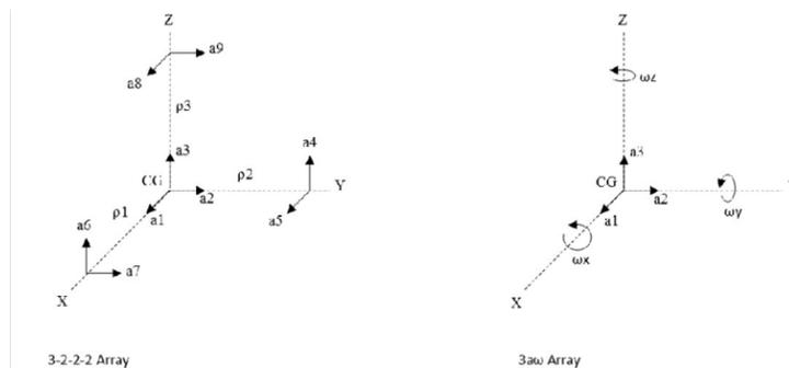
Figure 40: 3-2-2-2 Array of Accelerometers
