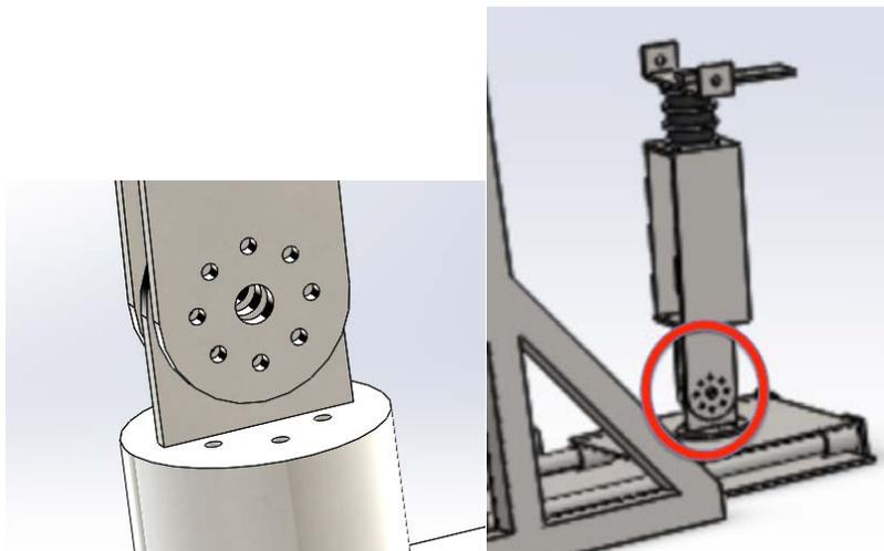
*Figure 24: Forward and Side Adjustment Points*
