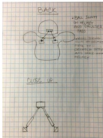
Figure 29: Initial Lift Support Design
