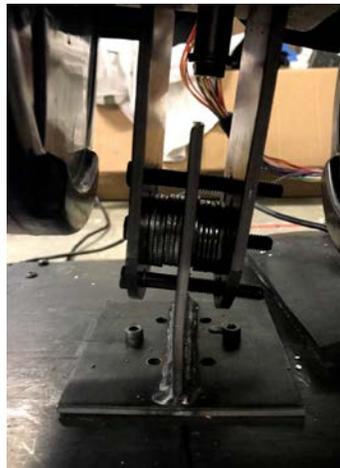
*Figure 64: Bent T-Bracket at the base of the Testing Dummy*
