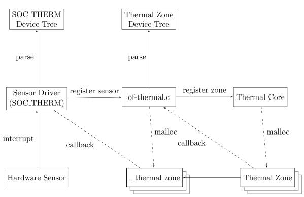
Figure 1.2: Diagram describing how SOC\_THERM and the thermal framework interact via of-thermal.
