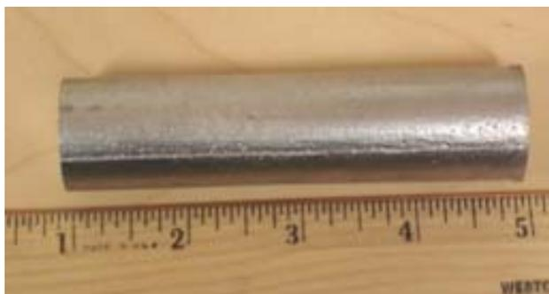
**Figure 3** Dimension of a Jominy End Quench bar of cast aluminum A356
