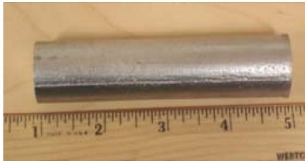
**Figure 1.** A cylindrical specimen of cast aluminum alloy A356
