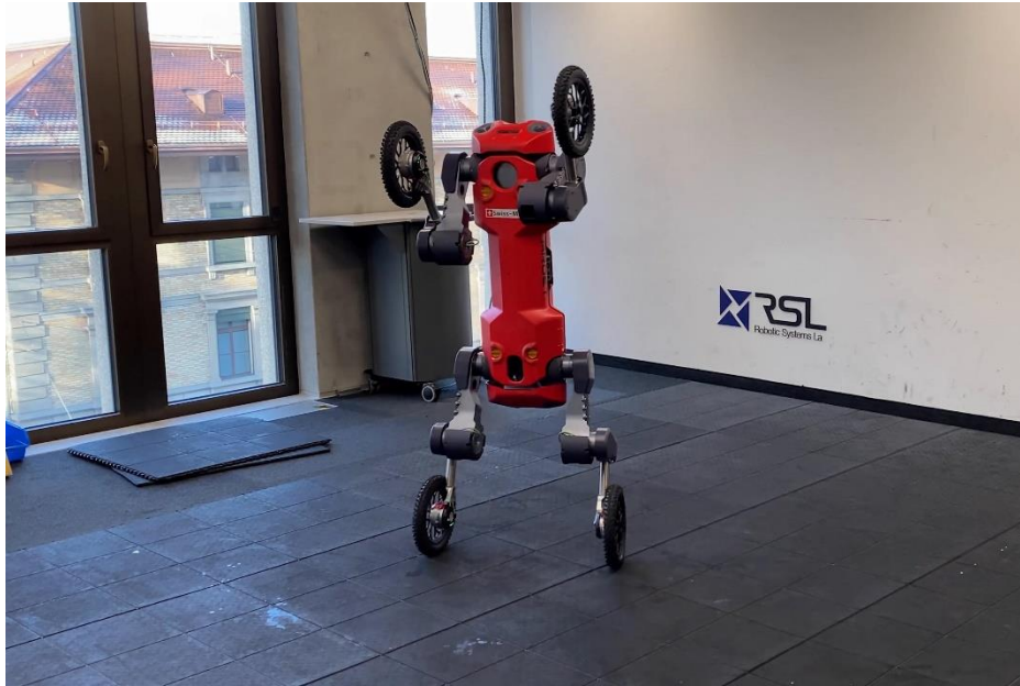
Figure 2: ANYmal as it stands in bipedal mode, assisted by wheels as feet
