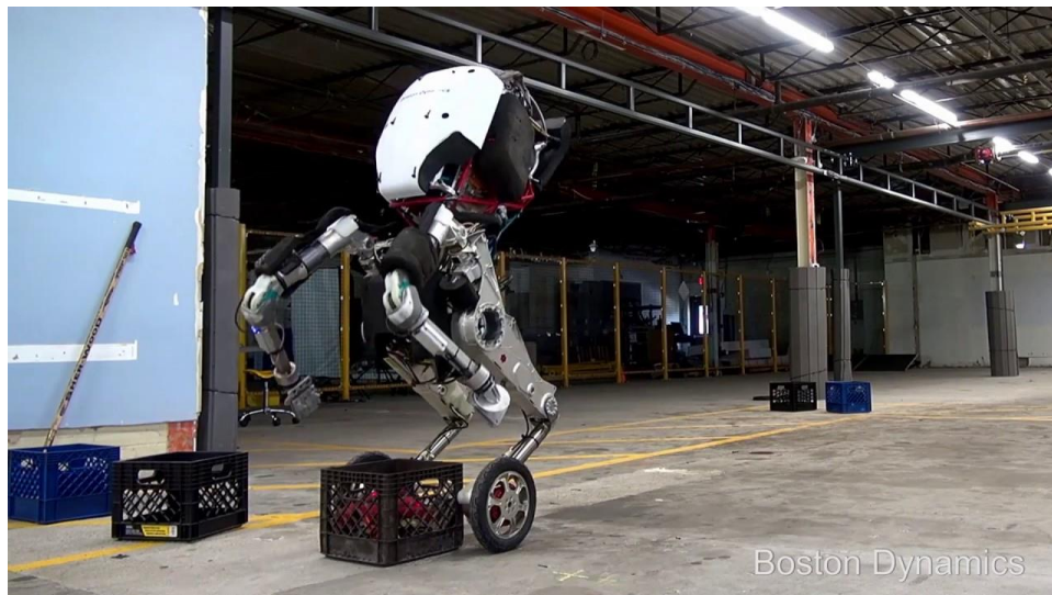
Figure 1: Boston Dynamics Handle as it attempts to pick up an example payload.
