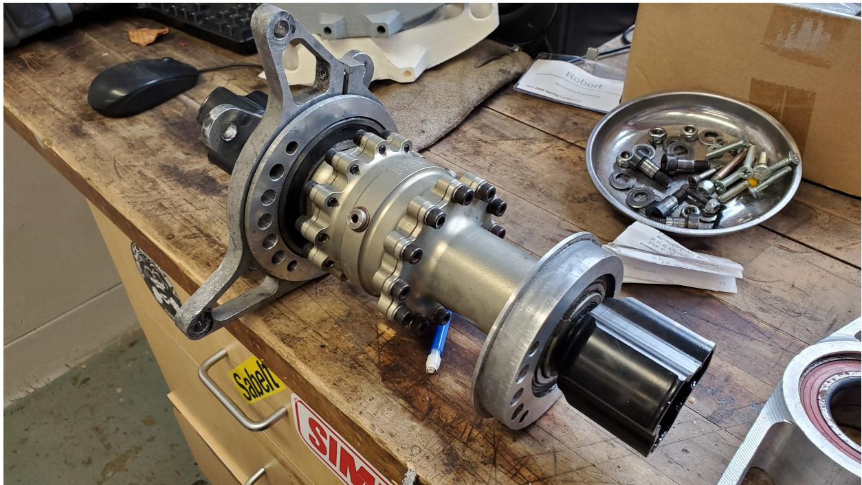
Figure 45: Drexler Differential With Mounting Collars
