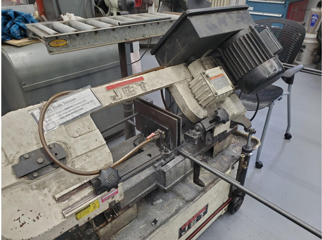
Figure 40: Control Arm Rods Being cut in the Horizontal Band Saw
