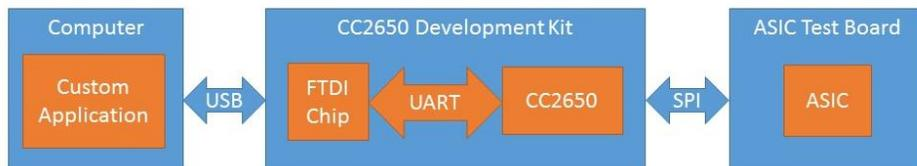
Figure 6: Second System Architecture
