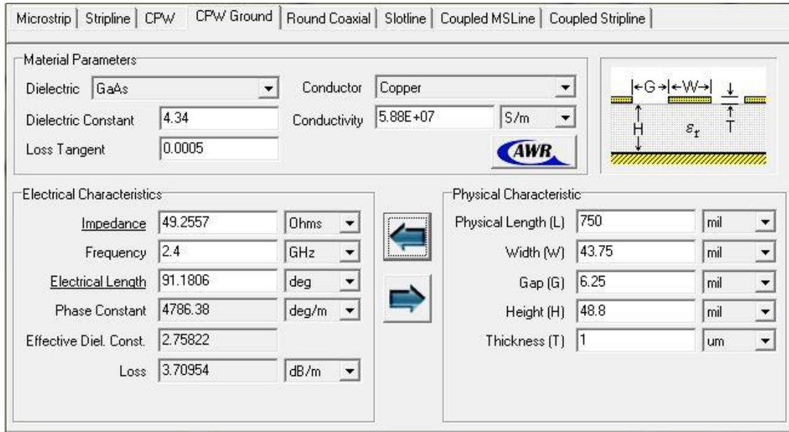
Figure 10: TX-LINE Microstrip Calculations
