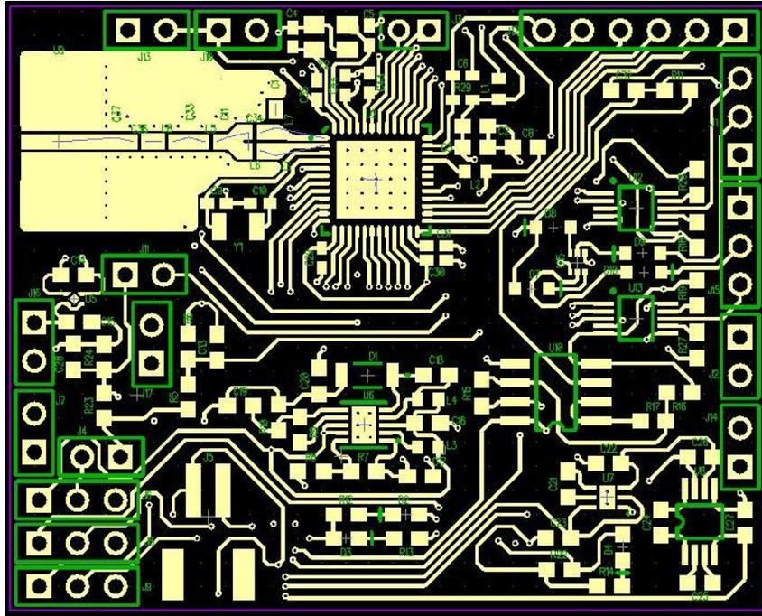
Figure 12: PCB Top Layout
