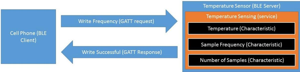
Figure 5: BLE Architecture Example - Write
