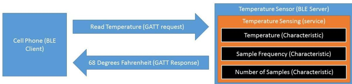
Figure 4: BLE Architecture Example – Read
