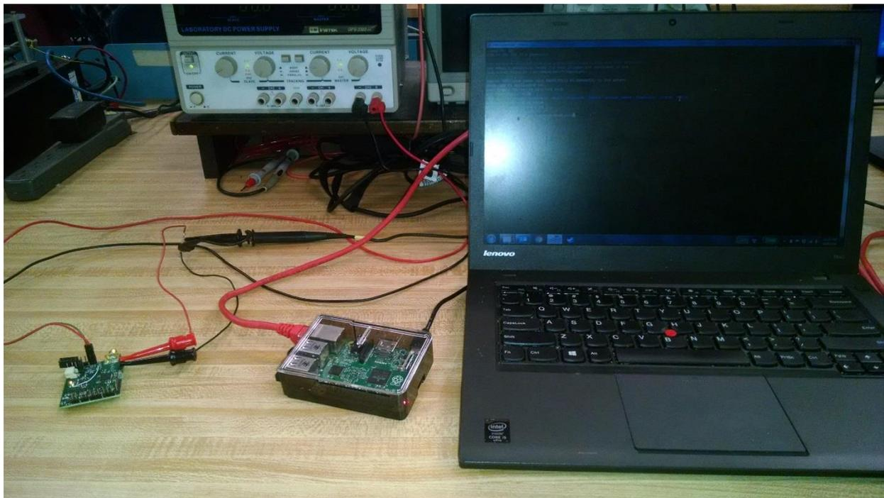
Figure 15: SSH Terminal Wireless Control
