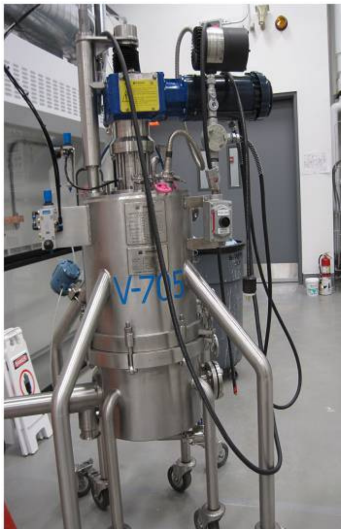
Figure 2: The 30 gallon Nutsche reactor used for filtering and cleaning of products.
