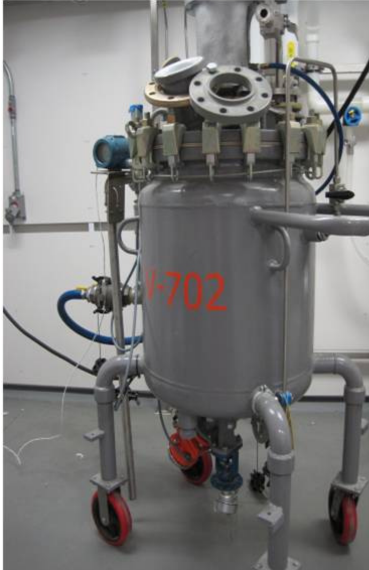
Figure 3: The 30 gallon stainless steel vessel used for the aqueous phase.
