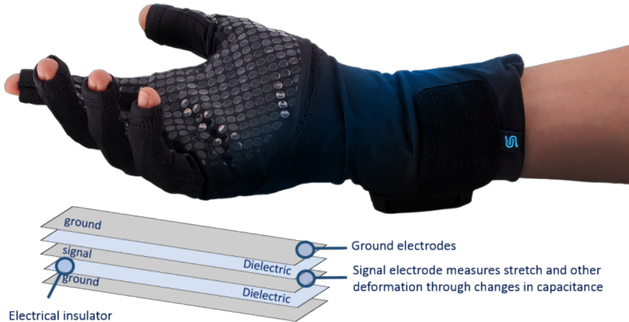
Figure 3.3: The StretchSense SuperSplay is an off-the-shelf data glove with capacitive curvature sensing. The curvature sensors are flexible layers that change capacitance when stretched.
