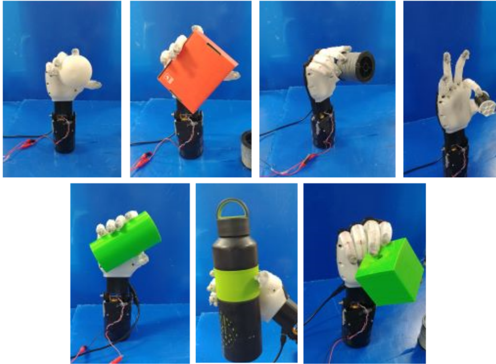
Figure 5.3: The fingers of the robotic hand are tendon driven and underactuated. The Ninjaflex fingers allow the fingers to conform to different shapes and perform a variety of grasps such as cylindrical, spherical, tripod, and pinch grasps.
