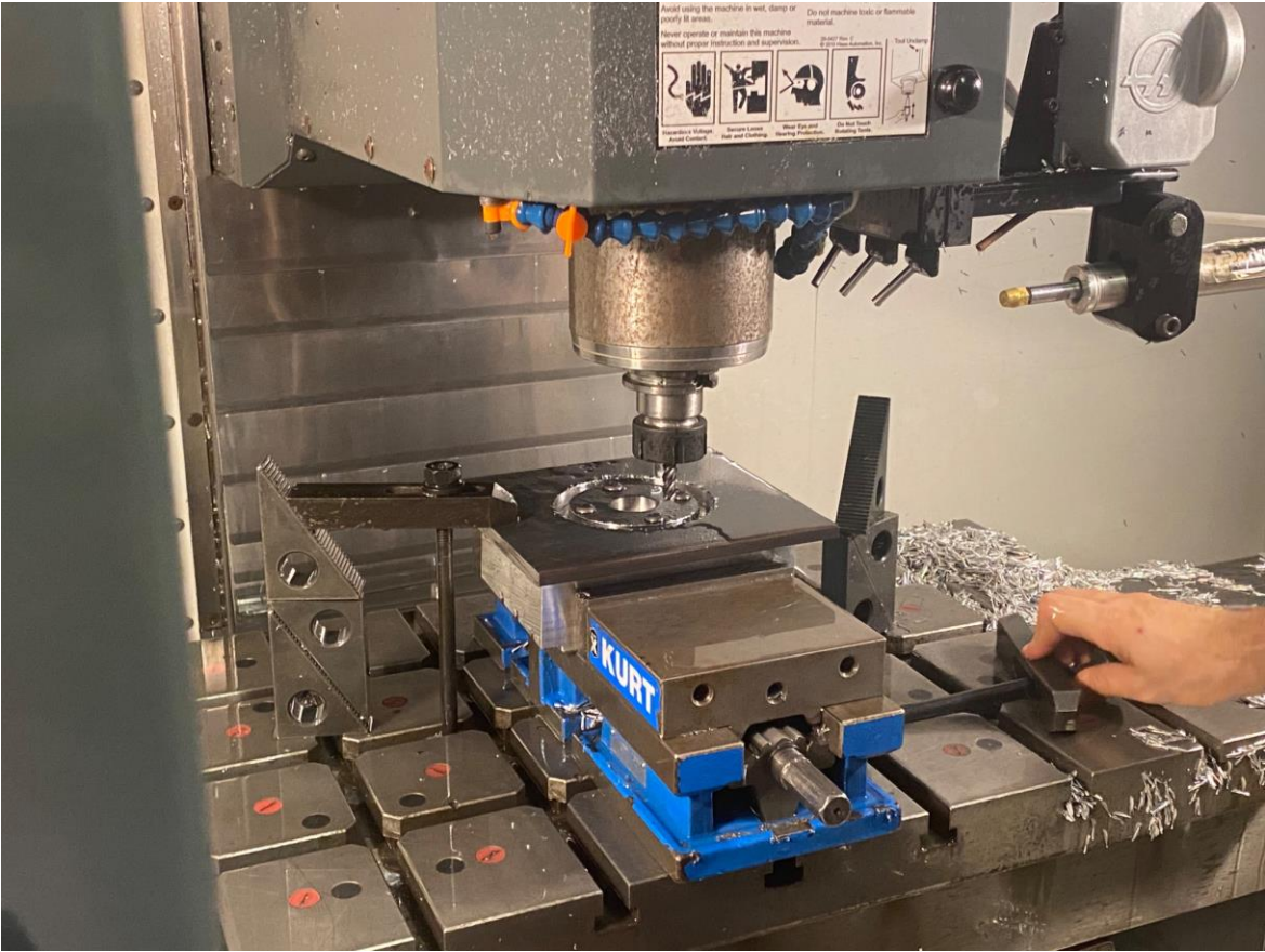
Figure 86. Circular Mounting flange after final operations on HAAS VM-2 Mill
