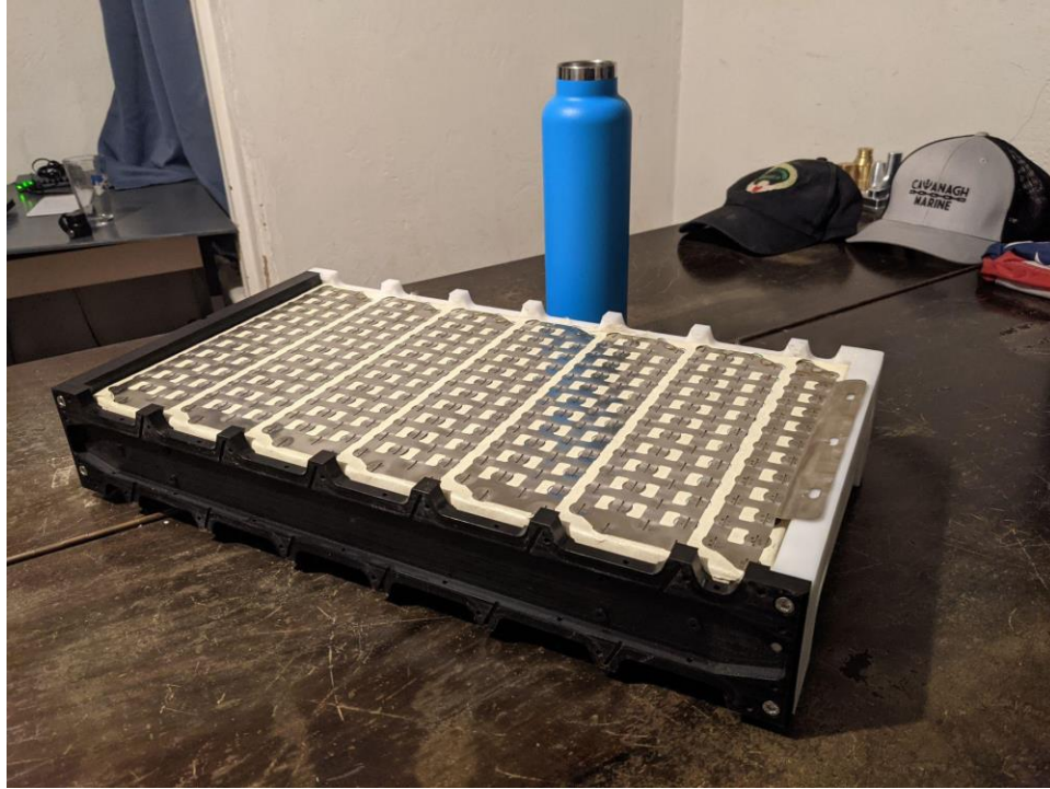
Figure 9. A Single “Beta Pack”, housed in a machined plastic housing.
