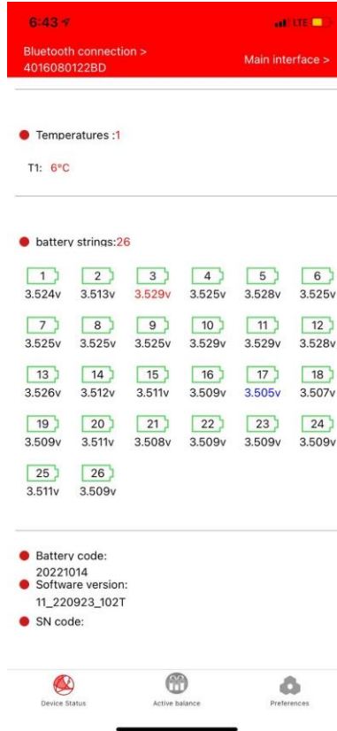
Figure 14. Second Page of Readout from one of the three Daly BMS systems.
