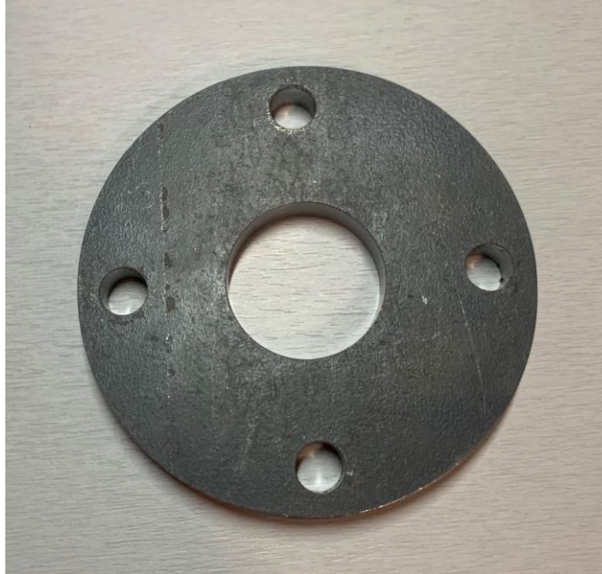
Figure 87. Fully machined Slip yoke mounting flange
