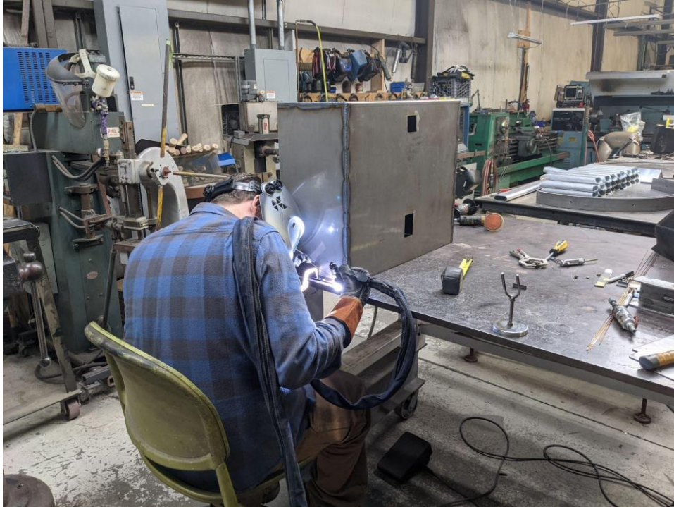
Figure 62. Charlie at ProShaper TIG welding the corners of the battery box.
