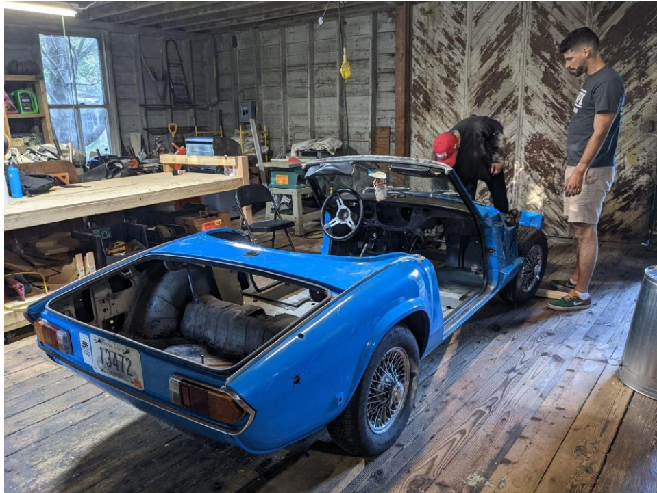
Figure 16. A photo of the car with the trunk lid and fuel tank removed
