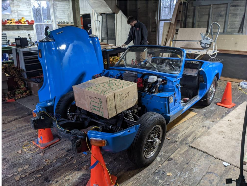
Figure 25. Initial testing of battery box sizing
