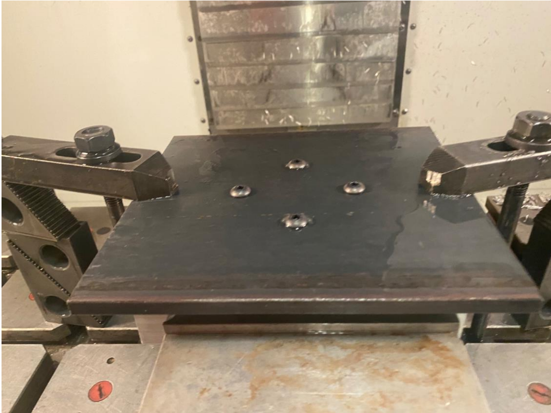
Figure 84. Setup of workpiece fully fixtured and ready for final milling operations.
