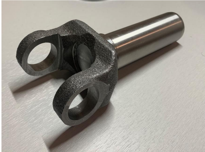
Figure 76. 2303-22 Slip Yoke compatible with T-50 transmission output spline
