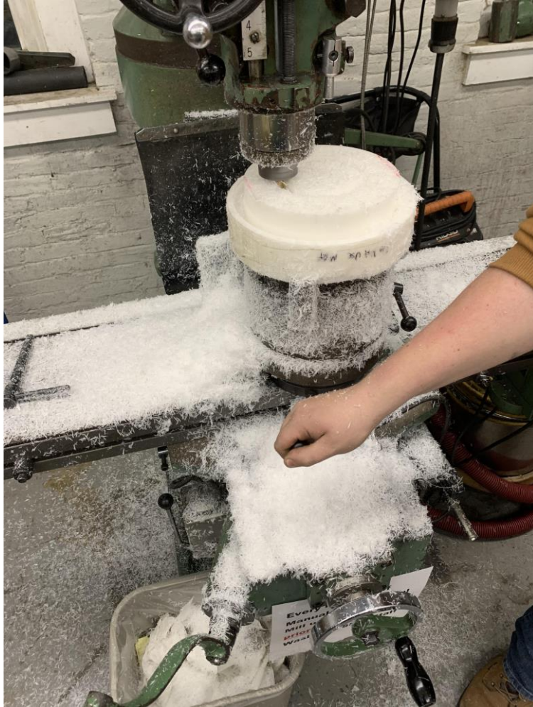
Figure 109. Motor Spacer Machining on a Manual Mill with a Rotary Plate Fixture
