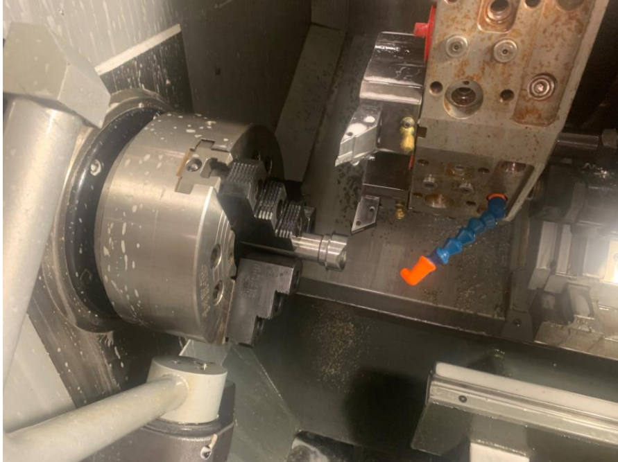
Figure 82. Reprofilng the slip yoke to a consistent OD of 1.260in” using a HAAS ST-30SSY Lathe
