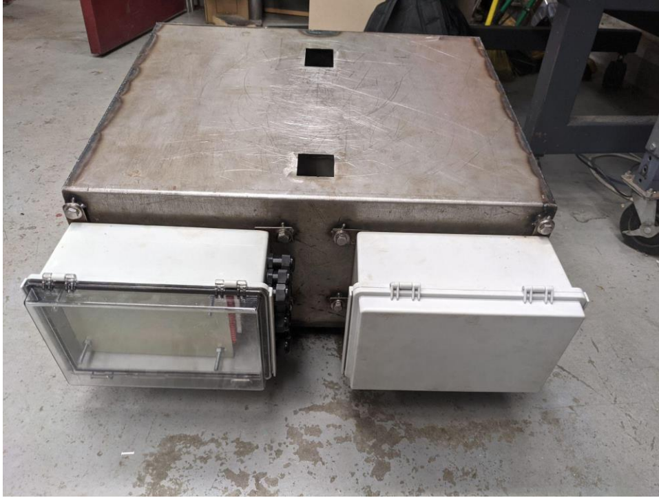
Figure 65. Initial Fitment of Junction Boxes 1 & 2 onto the battery box
