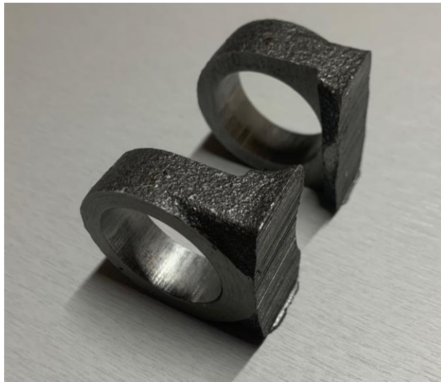
Figure 81. Rough Cut Material Removed from Yoke end of Slip Yoke
