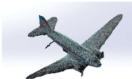
Figure 50: Image of the 3D scan taken of the DC-3 replica model. As can be seen the scanner did not create a full scan of the DC-3 itself and accidentally included geometry from surrounding objects.
