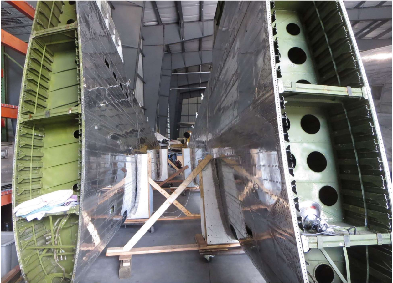
Figure 28: Image of both DC-3 wings detached during NEAM restoration process. [Personal Communication: email C. Cruff to J. Blandino, 1/16/23]
