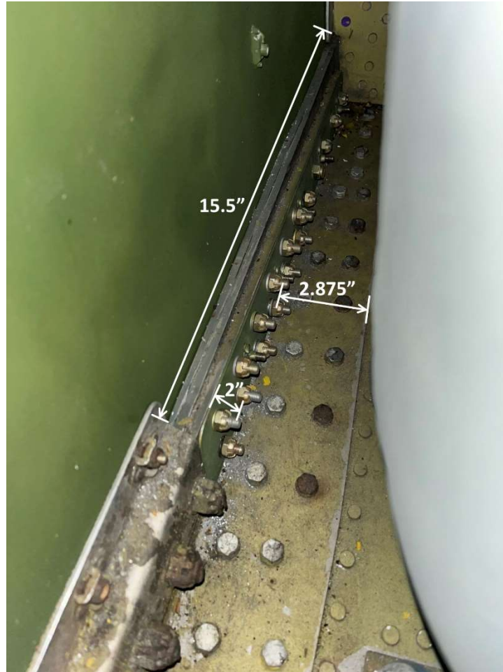
Figure 24: The above image was taken by the team of the internal wing structure, and annotations are visible to outline the dimensions of different sections.
