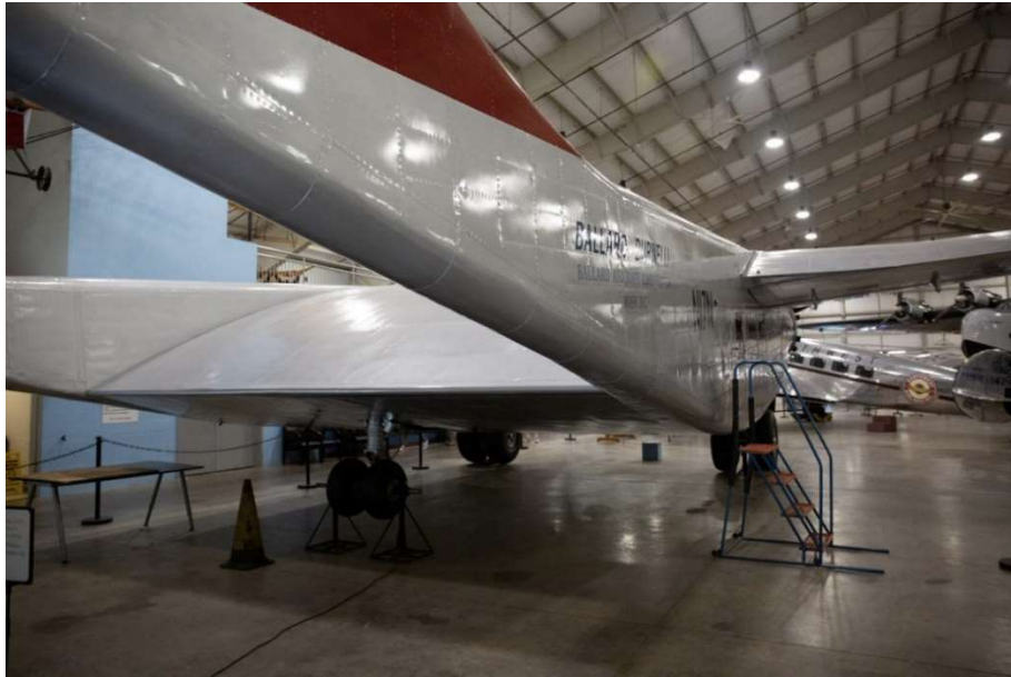
Figure 2: Rear-Right View of CBY-3 Loadmaster showing the trailing edge of the lifting body fuselage
