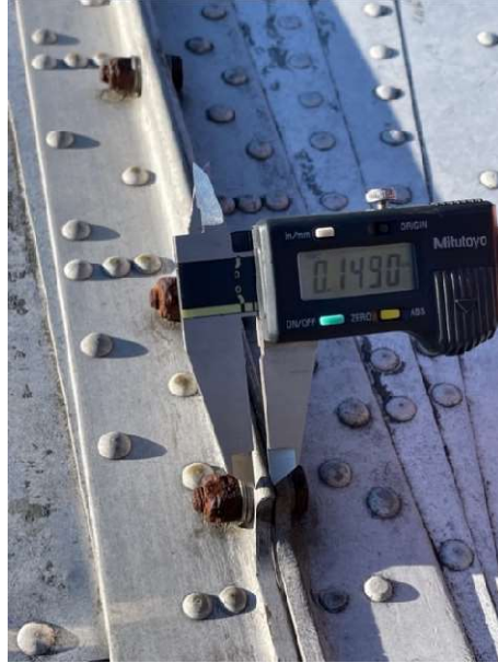
Figure 27: Measuring features using calipers on the detached DC-3 wing.
