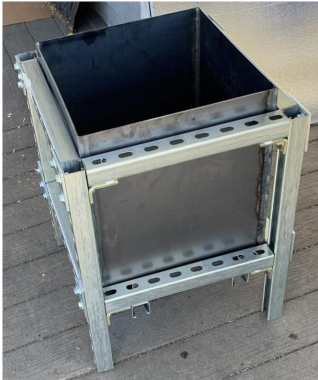
Figure A.3: The steel frame with the container intended to house the coils and water in.
