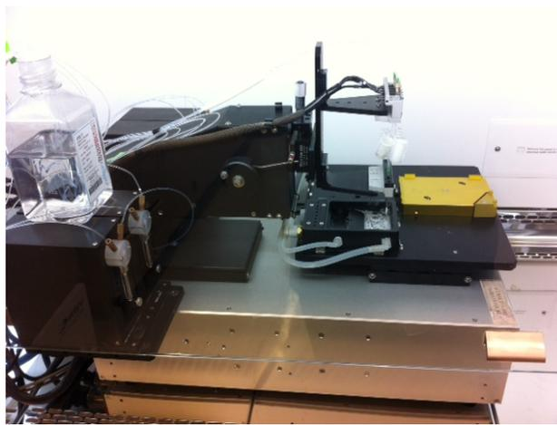
Figure 13 Digilab's commercial cell printer the Cell Jet
