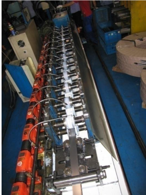
Figure 9: Roll Forming Process
