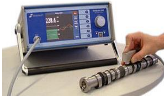
Figure 12: The Barkhausen noise equipment [25]
