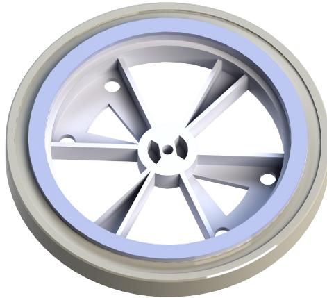
Figure 5.1: Base of the arm that connects to ROV. Four M5 screw holes, stability bearing on the outside, and servo horn attachment in the center.
