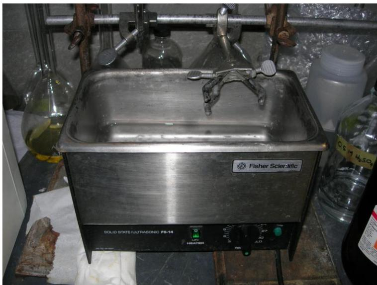
**Figure 10.** The Fisher Scientific Solid State/Ultrasonic FS-14 sonicator.
