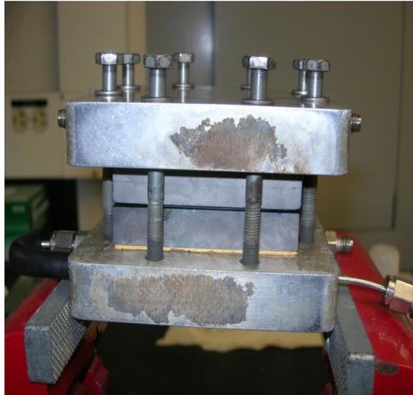
**Figure 16.** The fuel cell assembly.
