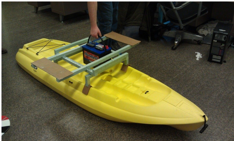
Figure 8: Foam and cardboard chassis mockup
