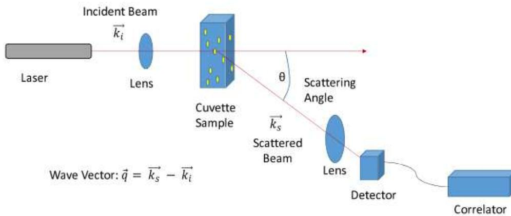
Figure 4-1: Light Scattering Components
