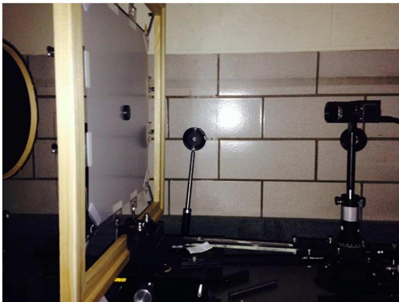
Figure 5-9: ARGOS Set-Up Portraying Camera, Beam Attenuator and Camera
