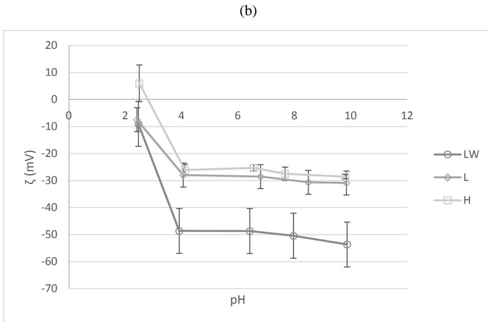
Figure 6-6: Zeta Potentials of Filter Media in Solutions of Varying Ionic Strengths (a) Sand and (b) Acid-Washed Sand (error bars represent standard deviation, n=4)
