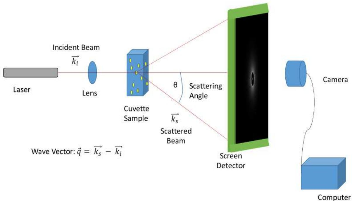
Figure 5-7: Components of the ARGOS Method
