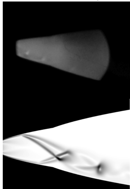
Figure 11: Comparison of schlieren (top) and Fluent (bottom) images of the density gradient.
