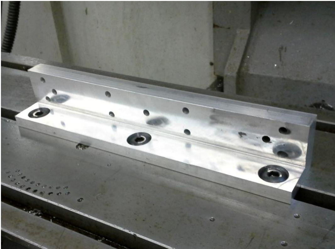
Figure 24: Fixture plate attached to CNC machine
