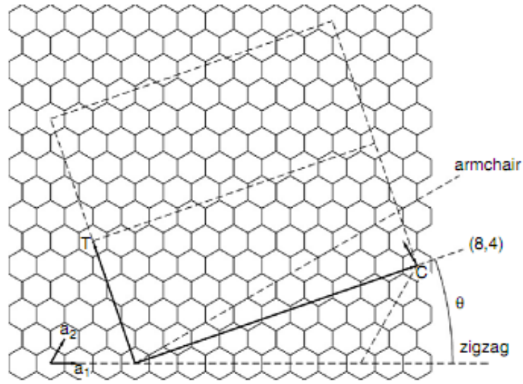
Figure 7: Rolling graphene nanosheet to form a SWCNT 27
