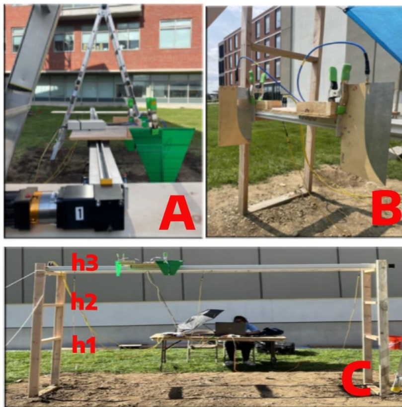
Figure 2: Log periodic antenna (co-pole) and ladder structure (Fig. A), Vivaldi antenna (cross-pole) wooden structure(Fig. B), Customized wooden structure with three heights h_1, h_2, h_3 (Fig. C)
