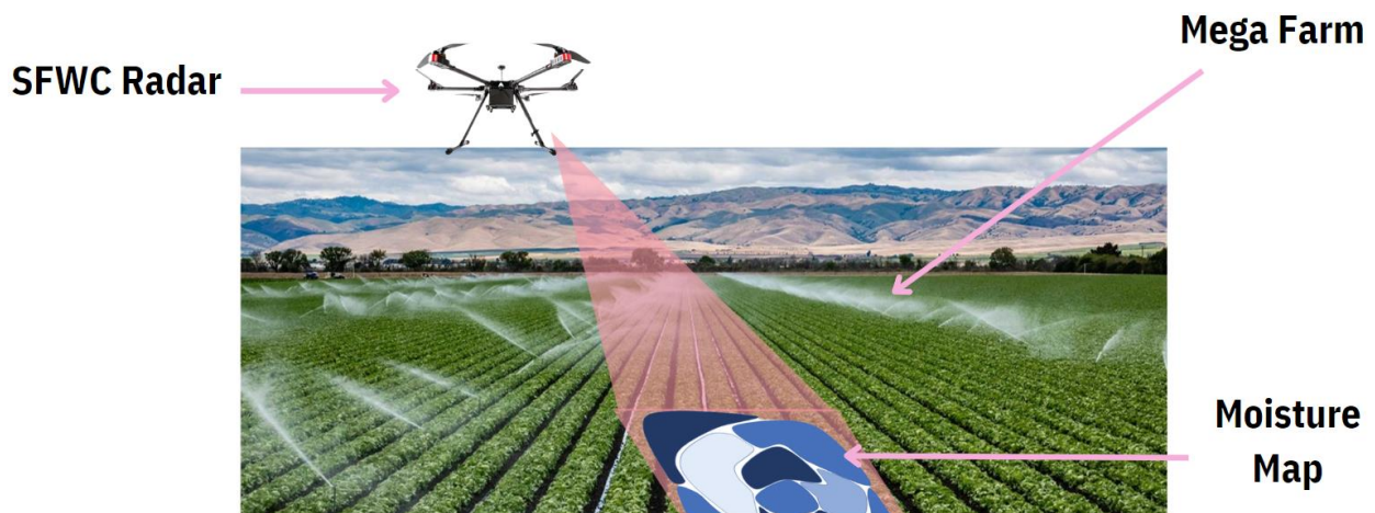
Figure 1: Image depicting an SFCW radar over a mega farm creating soil moisture maps.
