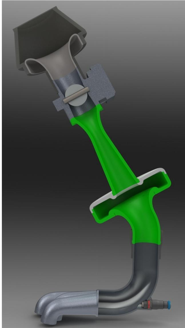
Figure 55. Cross Section of Prototype Intake Design with 1x Volume Plenum (colors as manufactured)
