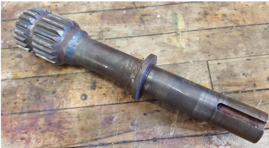
Figure 96. Steering shaft from the steering wheel to the steering box.
