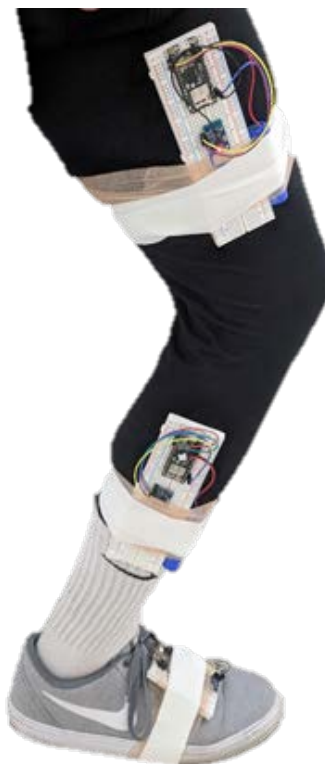
Figure 7.7. Three accelerometers attached to subject's lower limb at the center of mass of the thigh, shank, and foot.
