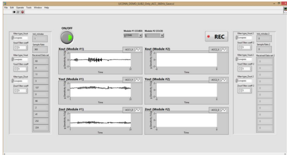
Figure 25: VI File Layout for Wireless Accelerometer
