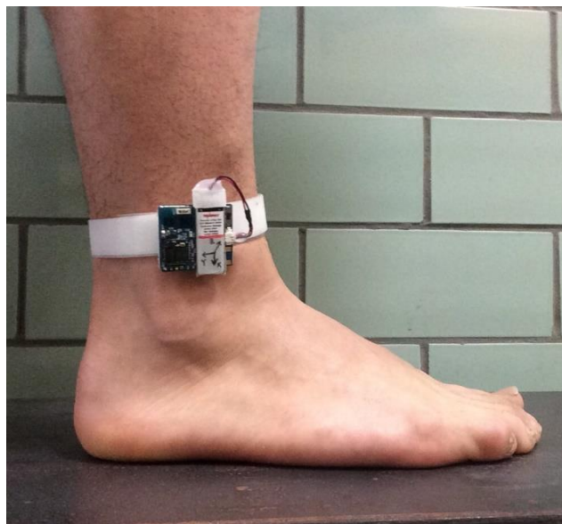
Figure 24: Wireless Accelerometer Setup
