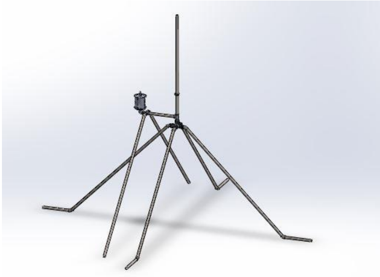
Figure 12: Turbine tower with motor mount
