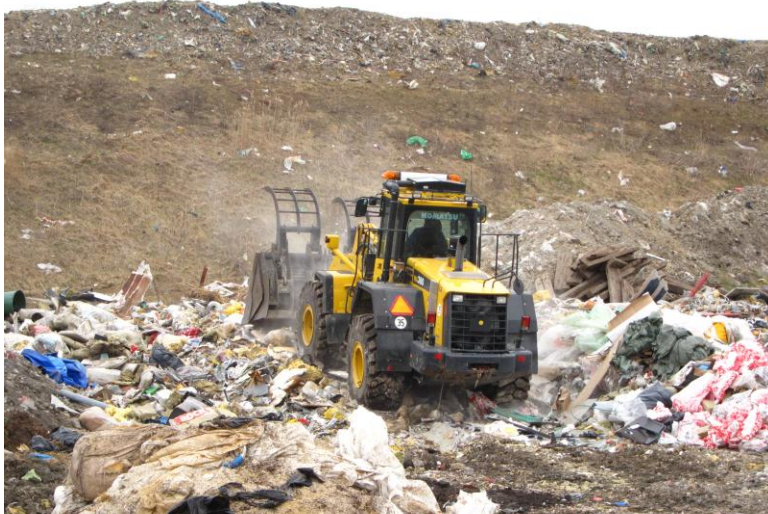
Figure 10: A front end loader compacting trash in a cell
