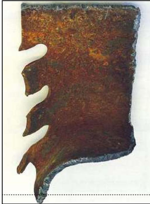
**Figure 9: Recovered Beam Stem Sample from WTC 5**
