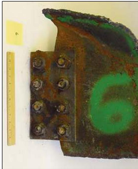
Figure 31: Shear Connection Specimen from WTC 5 (2 of 2)
