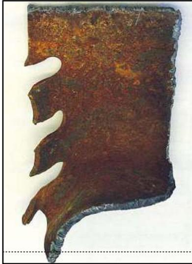
Figure 117: Recovered Beam Stem Sample from WTC 5
