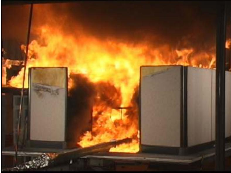
**Figure 41: Office Cubicle Assembly During Fire Exposure**
