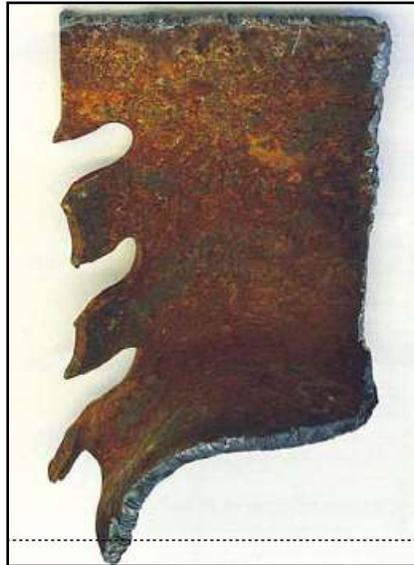
**Figure 59: Web Tear Out of a Beam Stem Web from WTC 5**
