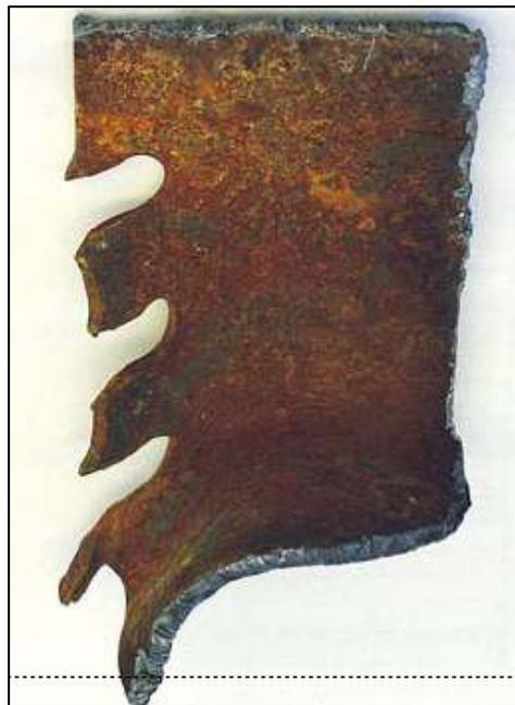
Figure 33: Failed Beam Stem Web Specimen from WTC 5
