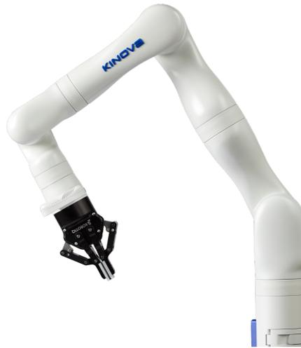
Figure 3.2: The Kinova Gen3 robot arm equipped with the 2f-85 Robotiq gripper [21].
