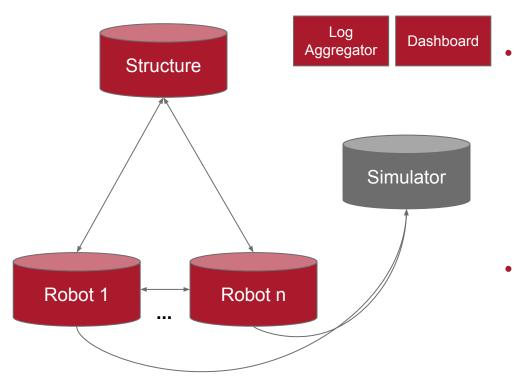
The architecture involves software for the robots, a custom simulator, the structure, as well as a dashboard to monitor progress Each entity communicates with
