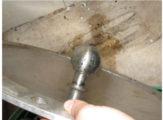
Figure 27: Low water consumption spray nozzle at Birra Puka. Taken on Nov. 21, 2019.
