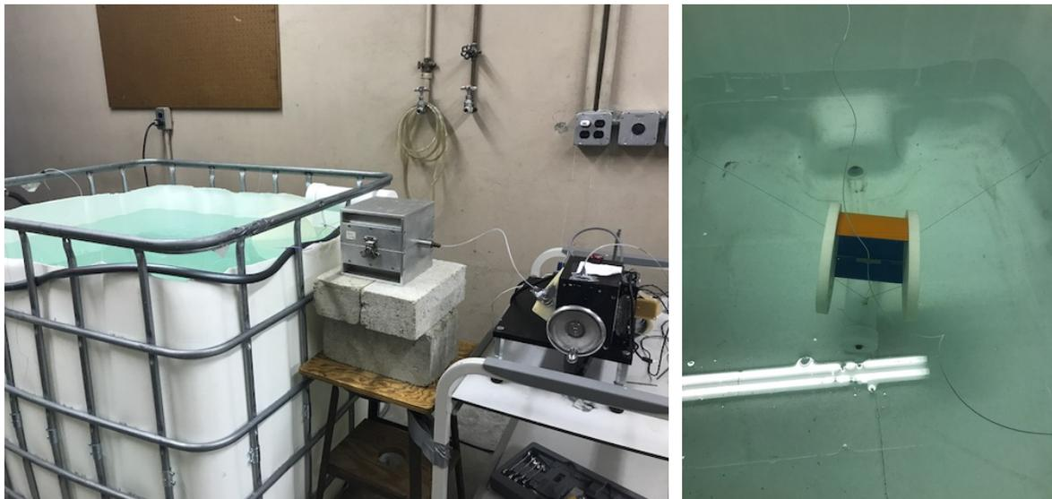
Figure 2.2: An image of the water tank, lead pig, afterloader, and catheter and wire running through it all (left). A top view of the tank, showing the film holder submerged in the water (right) (6).
