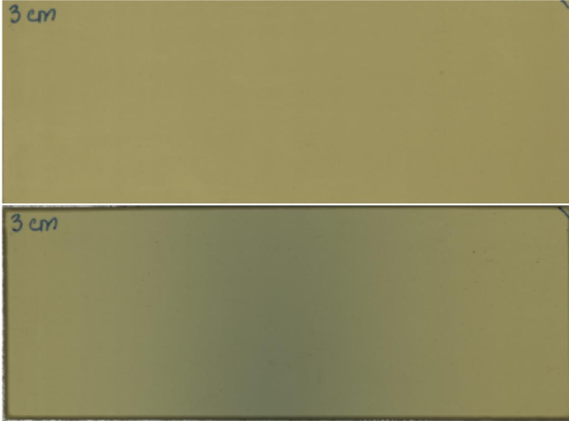
Figure 2.3: Scans of the Gafchromic film placed 3 cm from the seed before exposure (top) and after exposure (bottom) (6).
