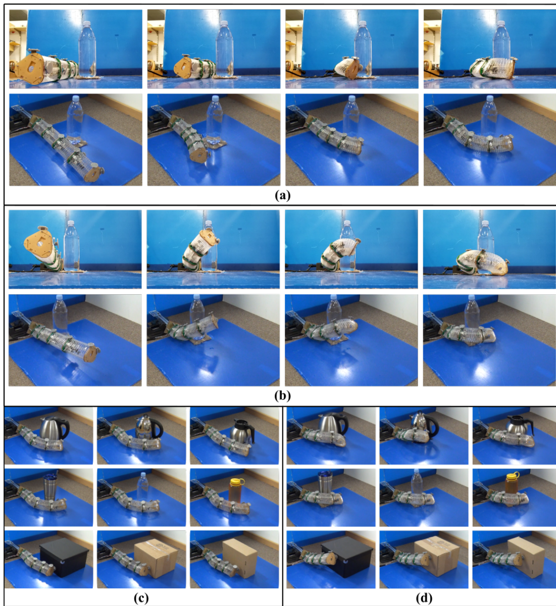
Figure 5.8: The motion snapshots of (a) planar and (b) spatial continuum wraps around the bottle, where the top and bottom rows show the motion of the same wrap from two view angles respectively. (c) Final configurations for the remaining objects with planar wraps. (d) Spatial wrap final configurations.
