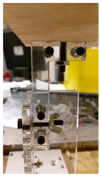
Figure 28: Heated bed L brackets
