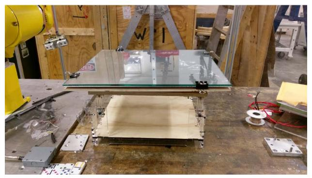
Figure 33: Final construction of heated bed
