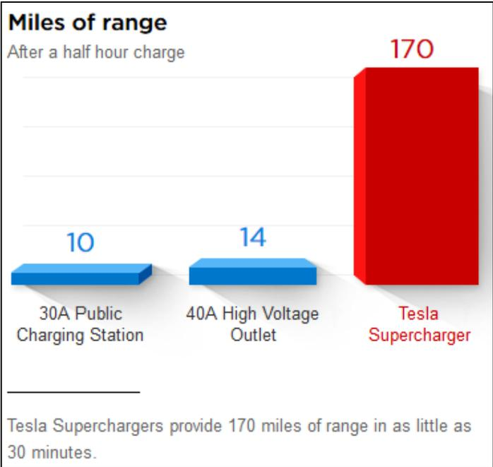
Figure 89: Tesla Supercharger vs. Other Chargers [56]
