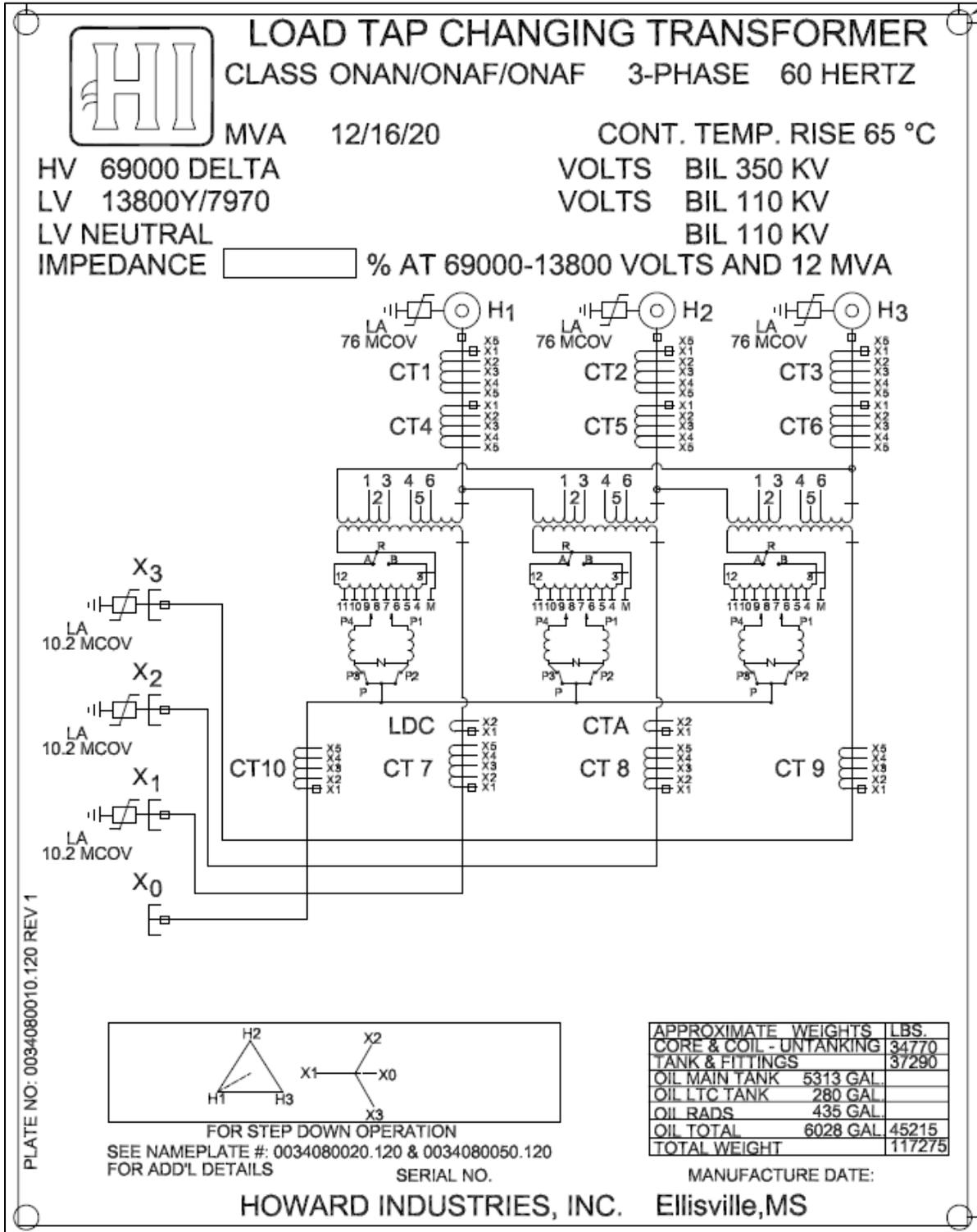
Figure 84: Transformer Specification 1
