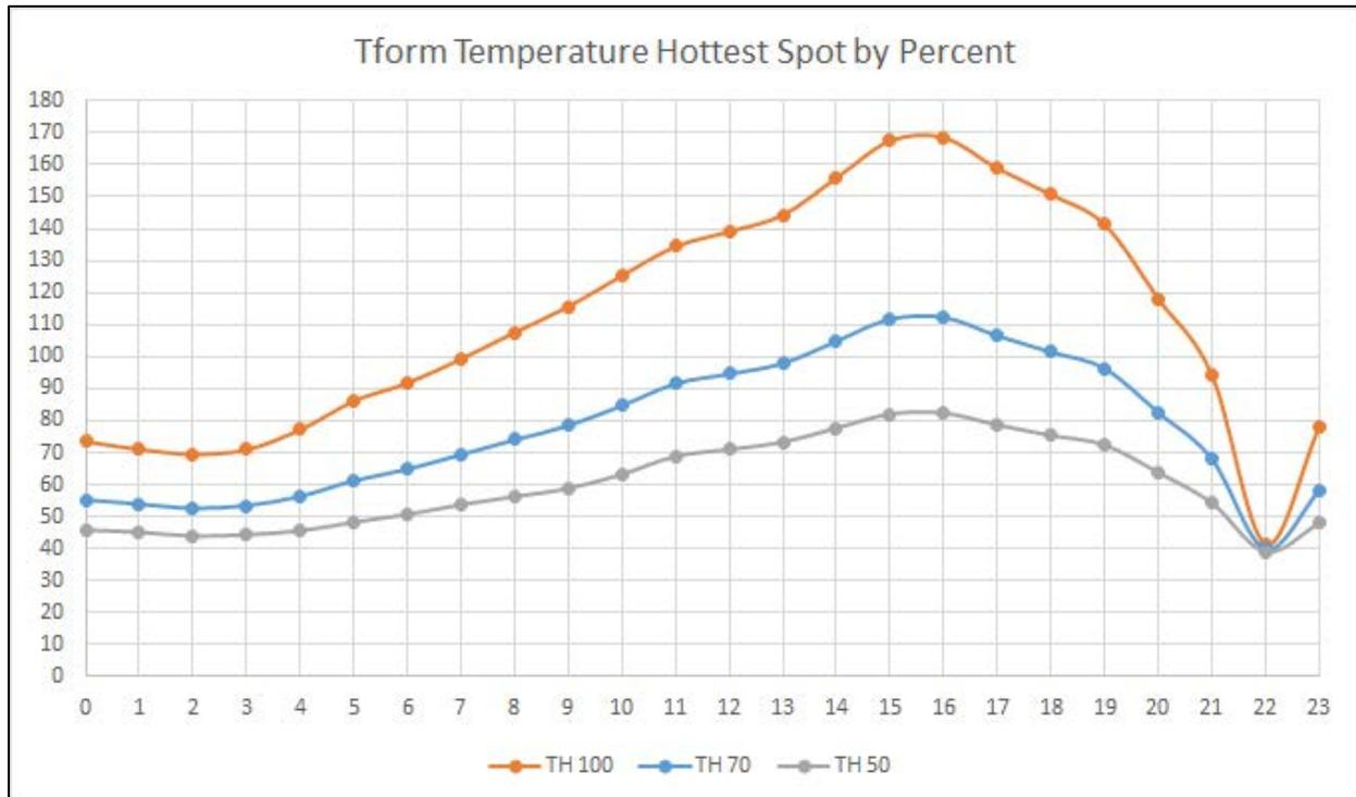
Figure 52: Hottest Spot for the 3 Loads in Table 13
