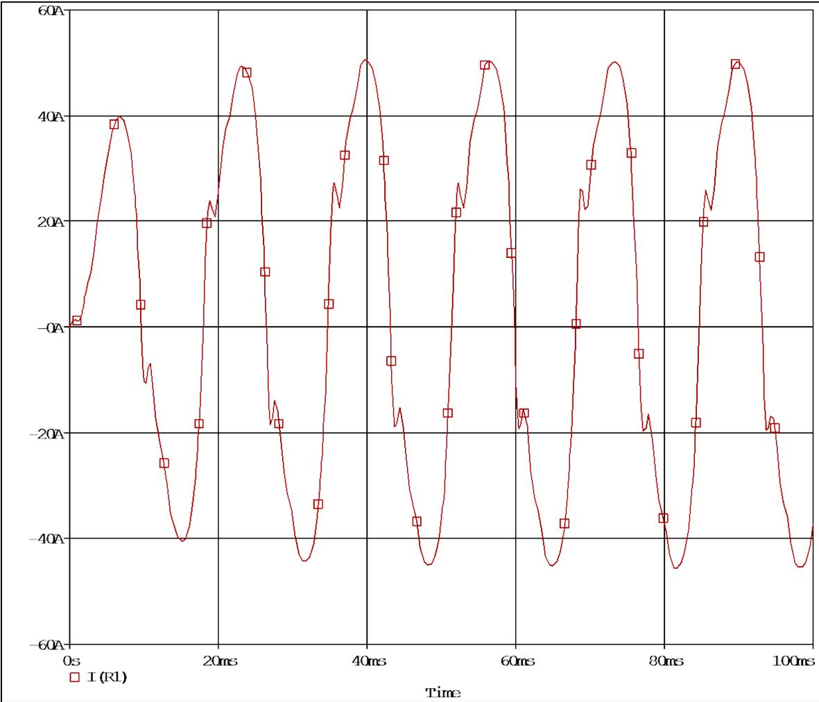
Figure 55: Single Car Charger from a Feeder Perspective
