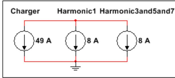
Figure 57: Battery Charger Model with Harmonics (Losses)
