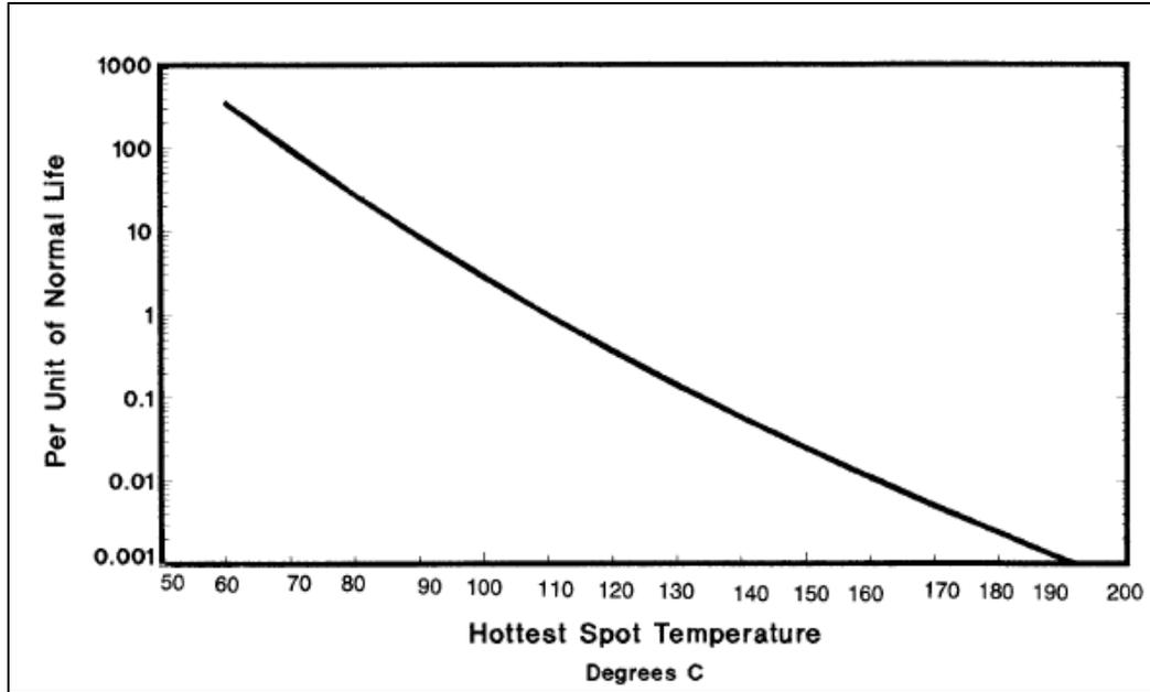
Figure 12: Per Unit Life as a Function of  $\Theta_H$  [33]
