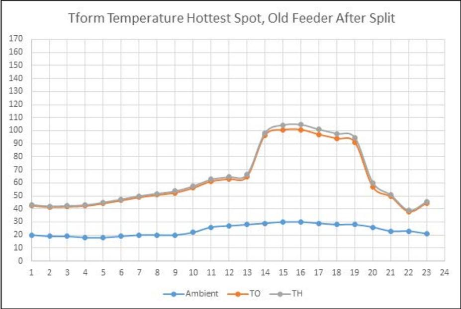
Figure 63: One Transformer, half of 65% Total Load, 100% Proliferation, 25 Years
