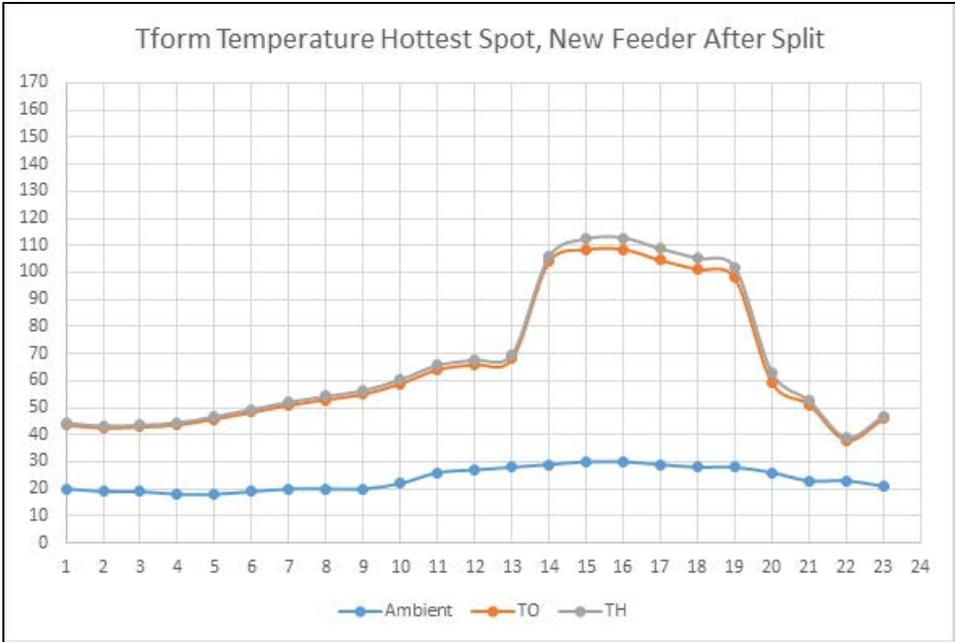
Figure 62: One Transformer, 35% Total Load, 100% Proliferation, 25 Years
