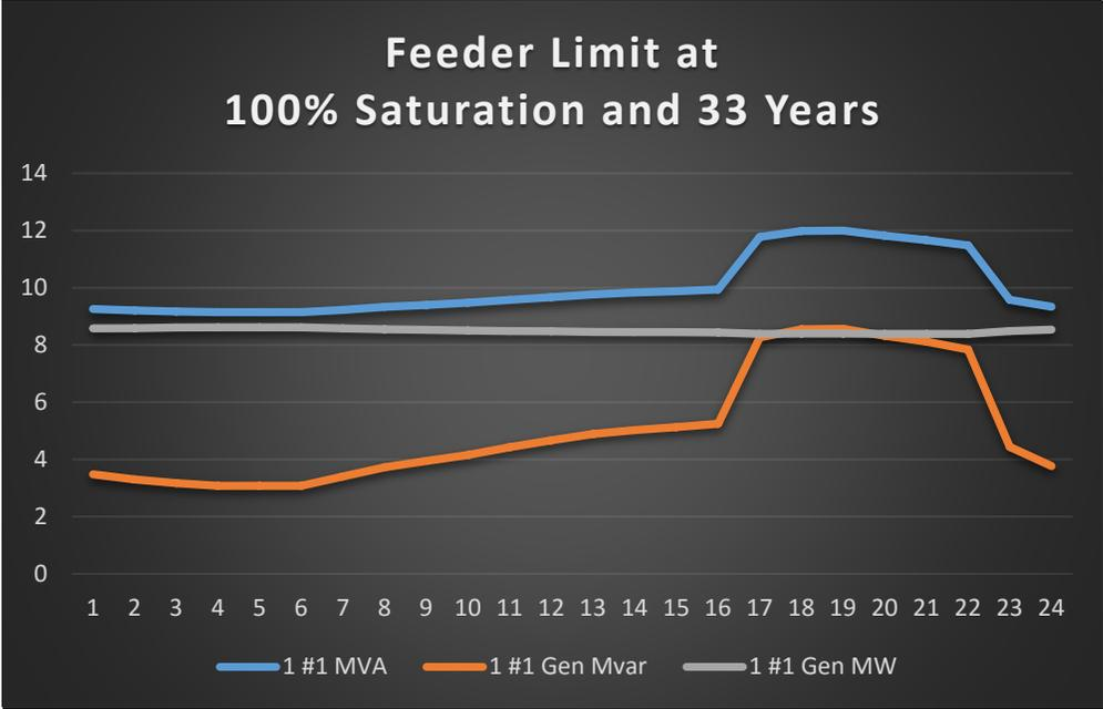
Figure 46: Feeder Limit with Feeder Storage at 100% Saturation and 33 Years
