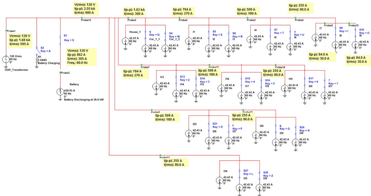
Figure 69: All cars charging at peak current draw, battery discharging
