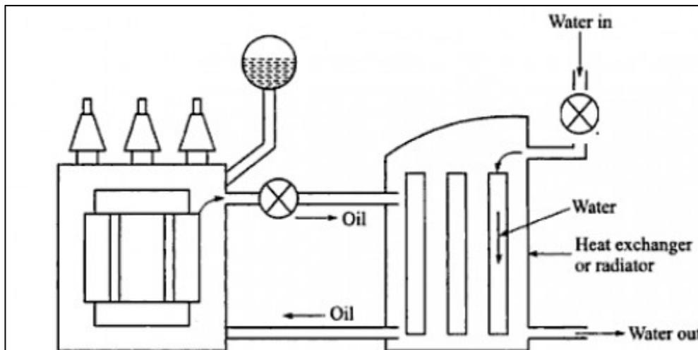
Figure 83: OFWF Cooling Method [53]
