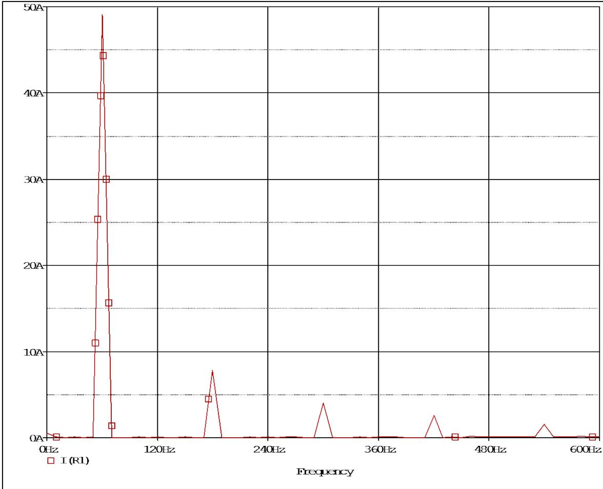
Figure 56: Fourier Response of One Car Charger from Feeder Perspective
