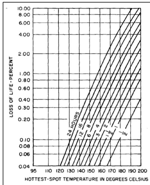
Figure 14: Summary of Percent Loss of Life Behavior as Function of Hottest Spot Temperature [33]
