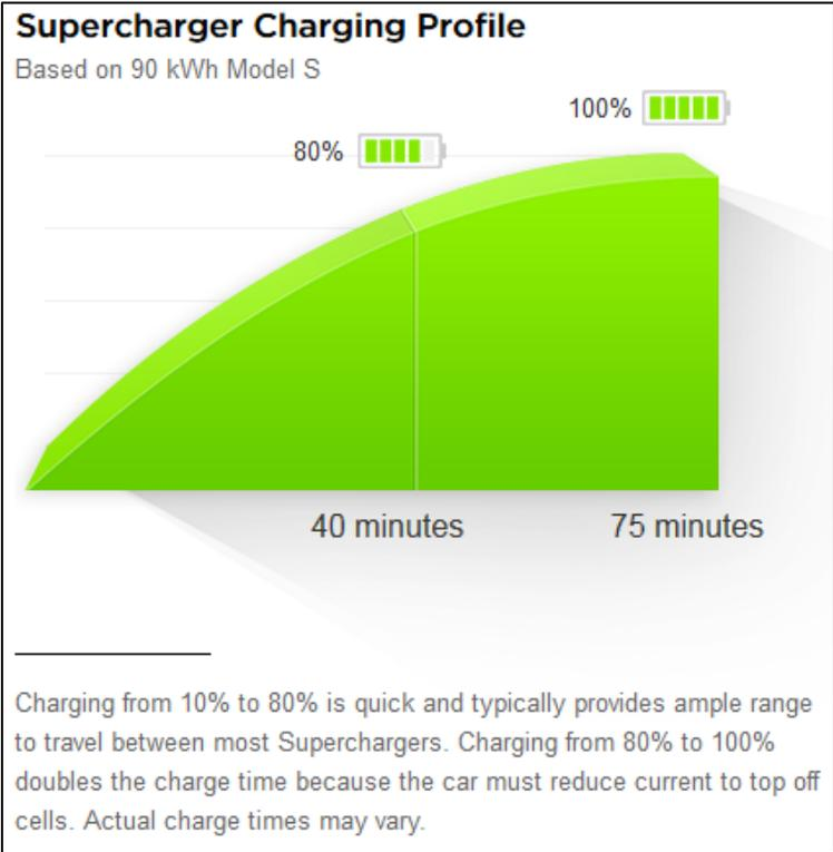
Figure 90: Tesla Supercharger Charging Profile [56]
