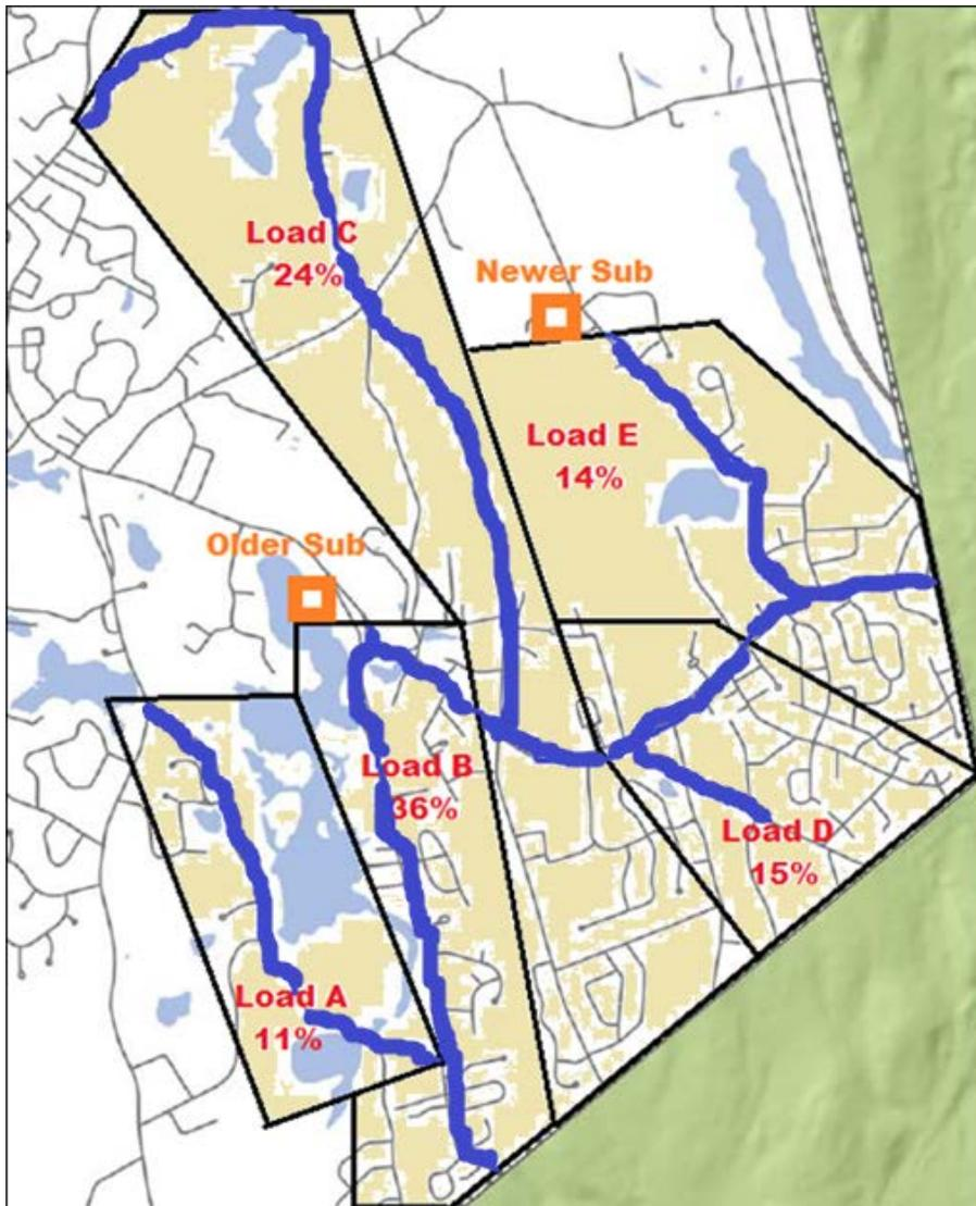
Figure 2: Annotated GIS Map of the Sample Feeder
