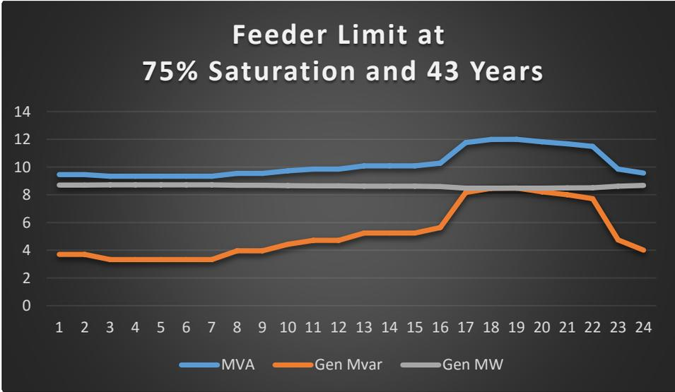
Figure 49: Feeder Limit for Micro-Grid Solution at 75% Saturation and 43 Years
