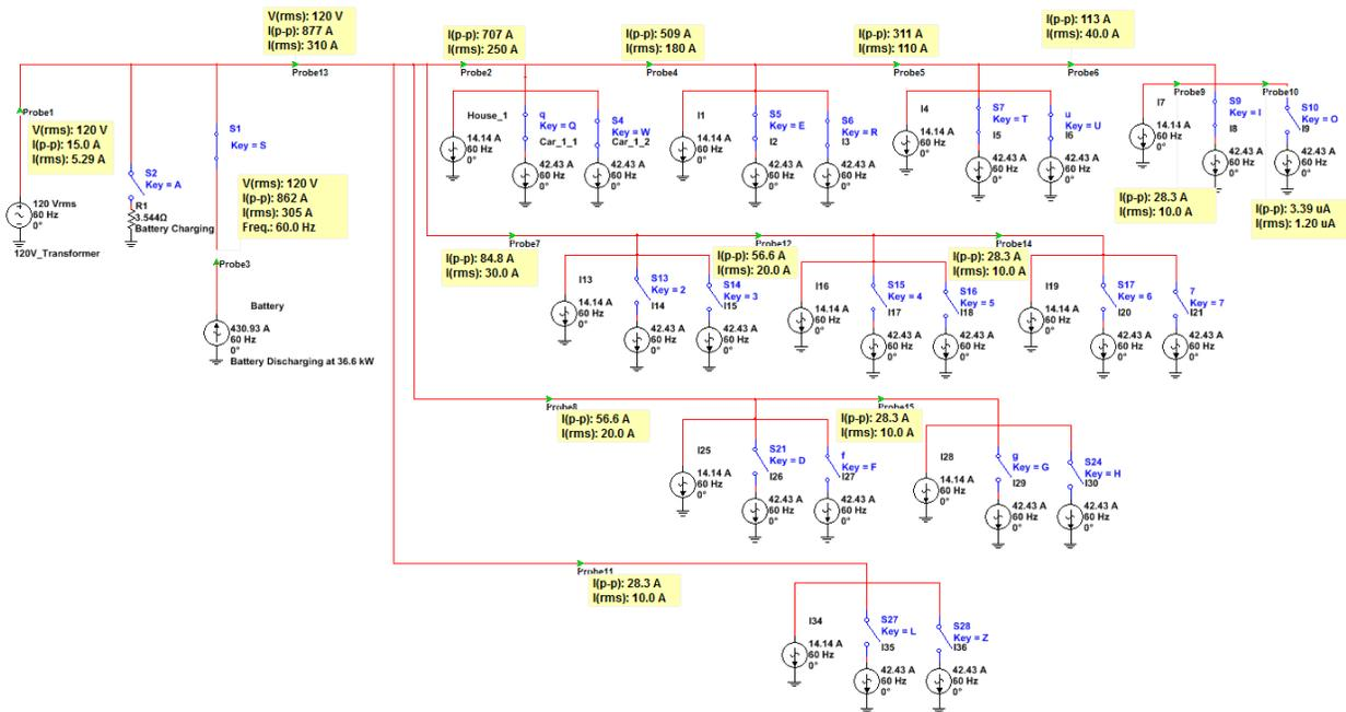
Figure 73: Seven cars charging at 10 A house current draw, battery discharging
