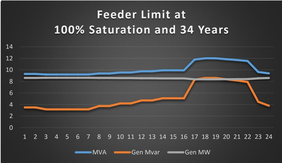
Figure 50: Feeder Limit for Micro-Grid Solution at 100% Saturation and 34 Years
