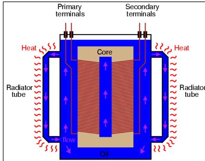
Figure 78: Distribution Transformer Cross-Section [47]
