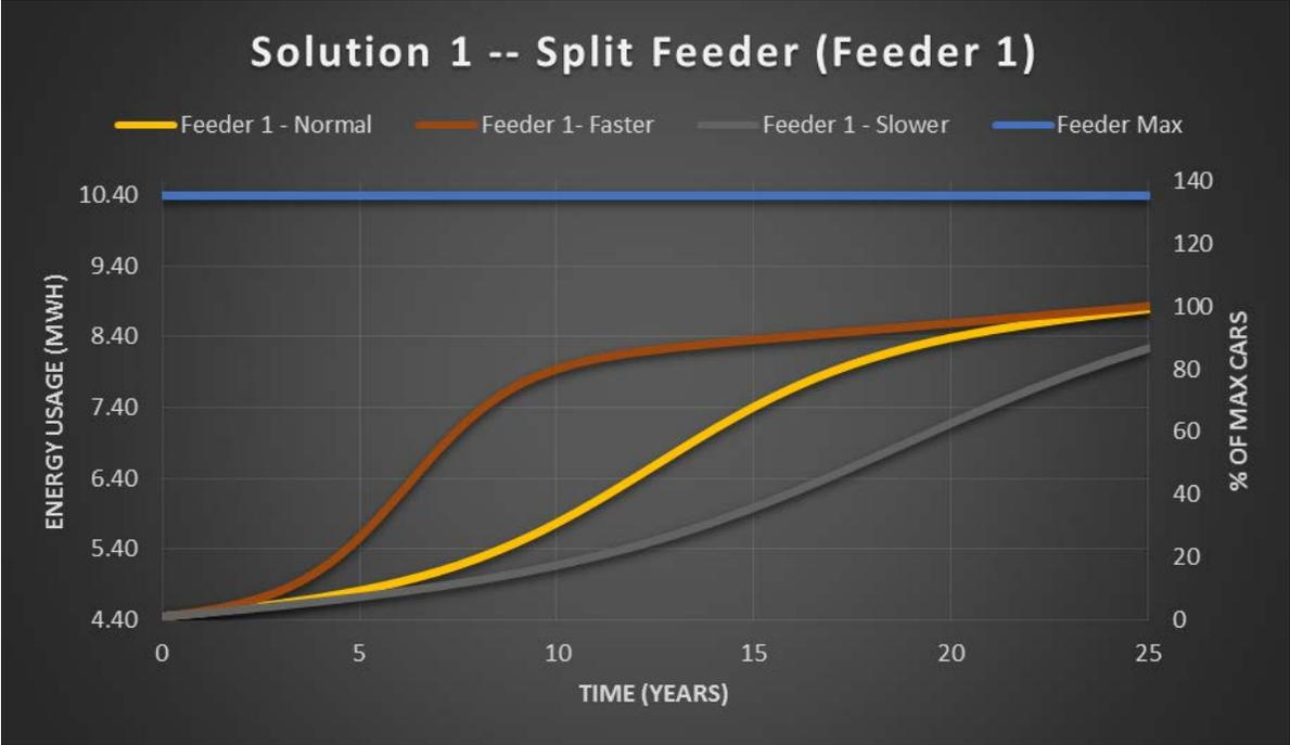
Figure 64: Solution 1 – Older Feeder S-curve with Feeder Maximum After Splitting
