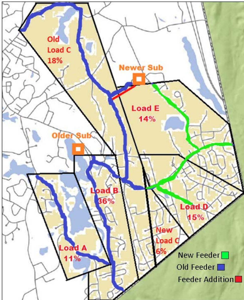
Figure 4 – Split Feeder Solution for Fast Proliferation
