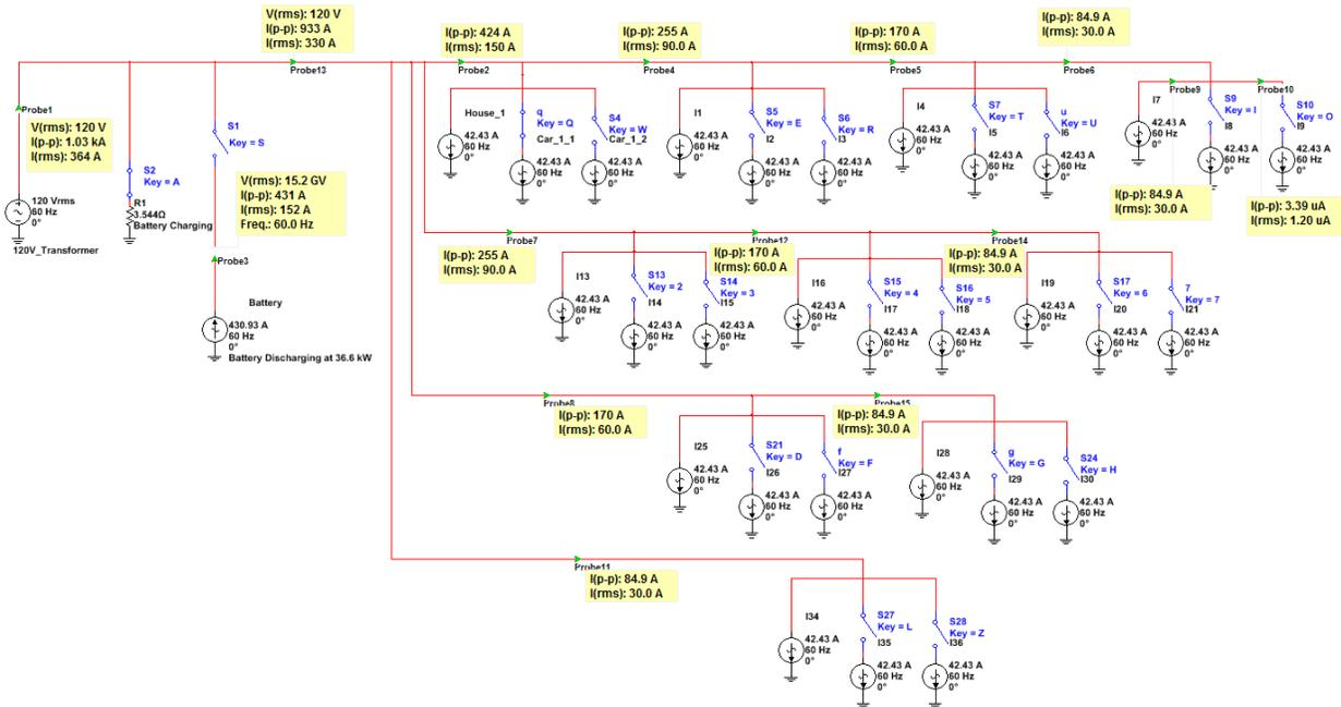
Figure 72: One car charging at peak current draw, battery discharging
