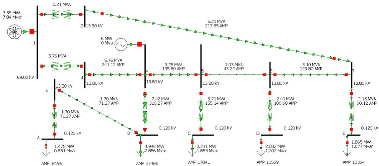
Figure 67: PowerWorld model – Peak Power Demand with the Feeder Battery Connected
