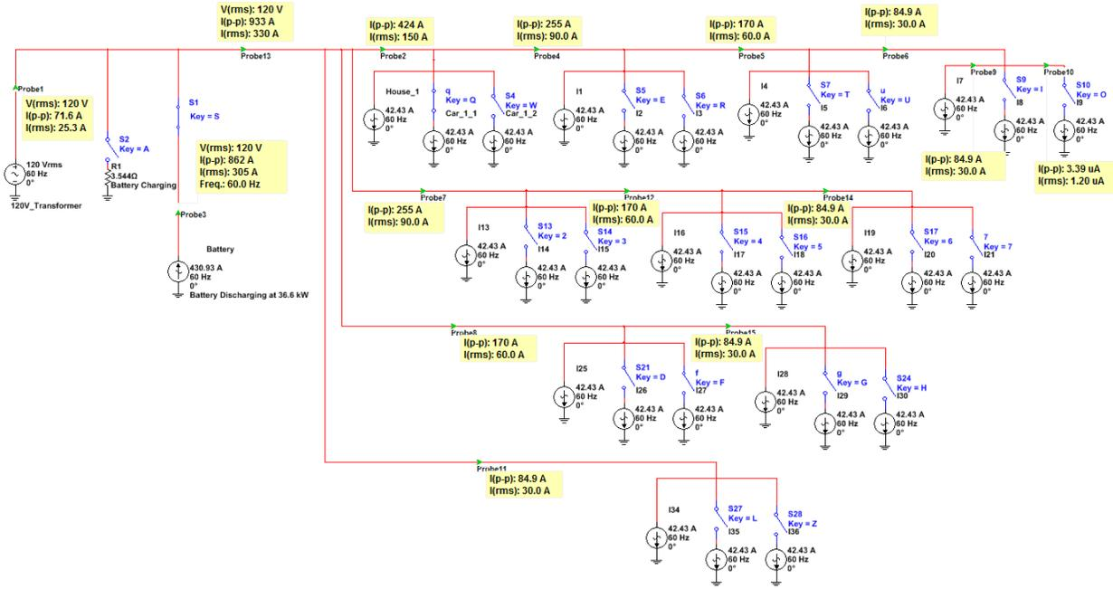
Figure 71: One car charging at peak current draw, battery charging
