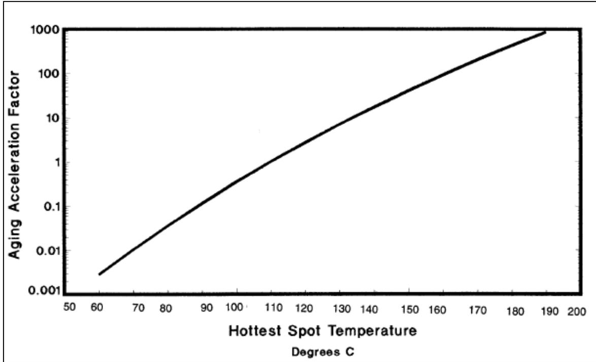
Figure 13: Aging Acceleration Factor as a Function of  $\Theta_H$  [33]
