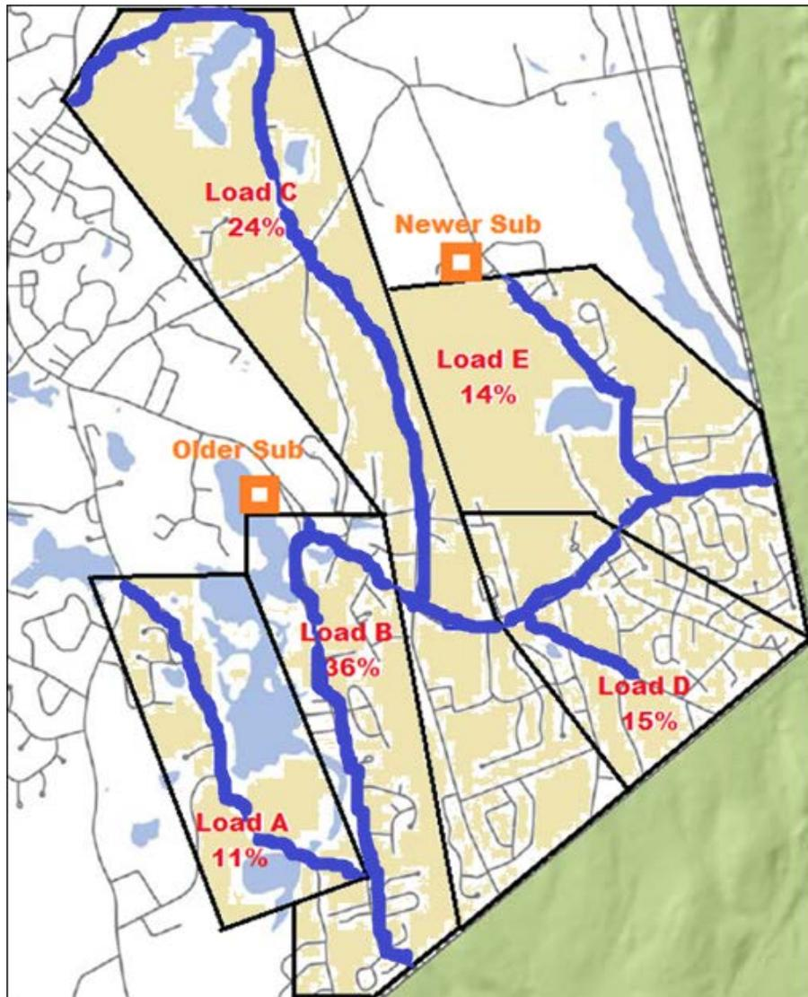
Figure 15: Annotated GIS Map of the Sample Feeder
