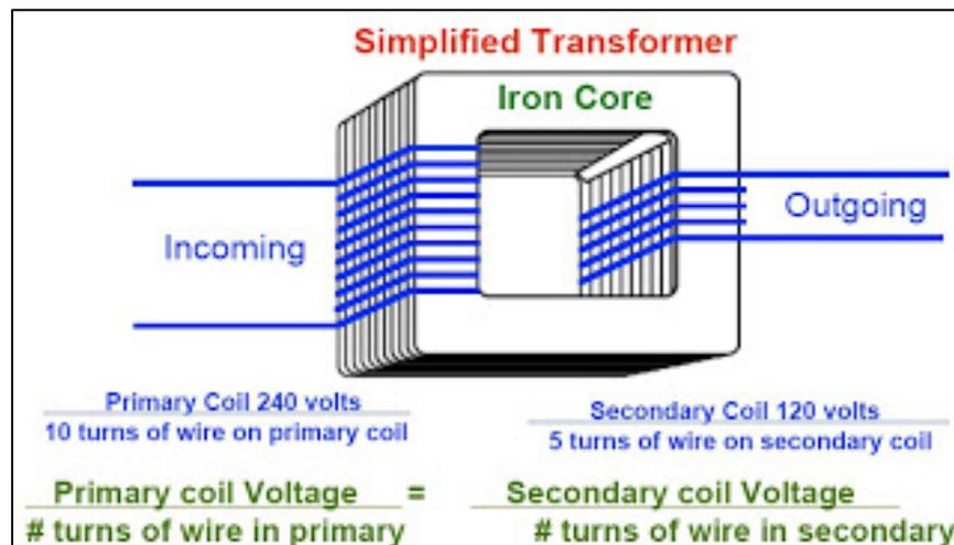
Figure 77: Transformer Basic Operation [44]
