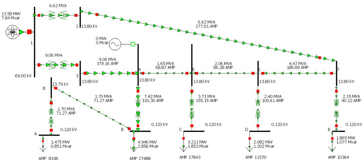
Figure 66: PowerWorld model – Peak Power Demand with the Feeder Battery Disconnected
