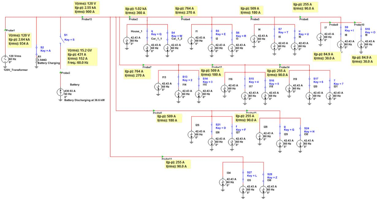
Figure 70: All cars charging at peak current draw, battery charging
