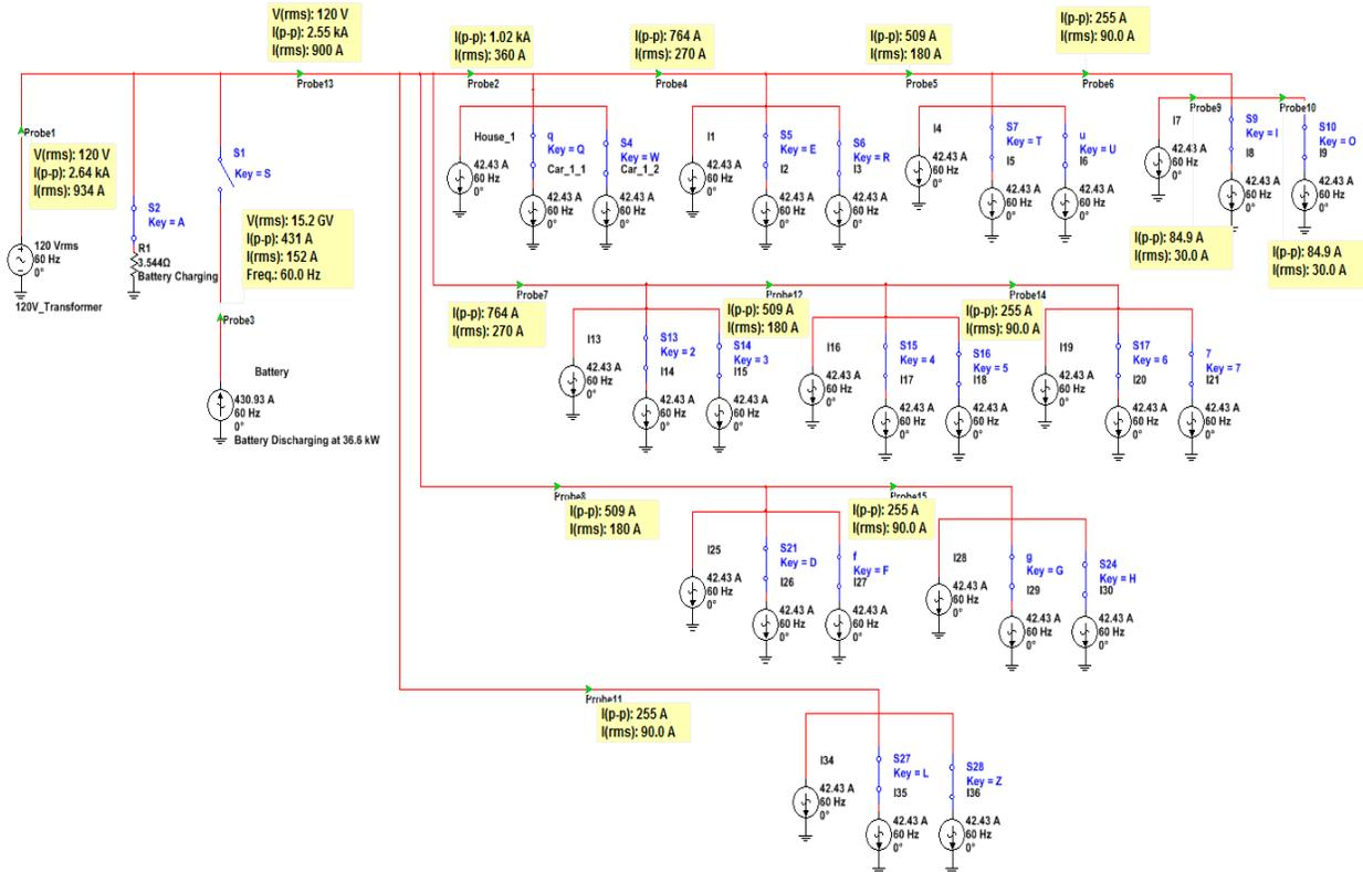
Figure 6: All cars charging at peak current draw, battery charging
