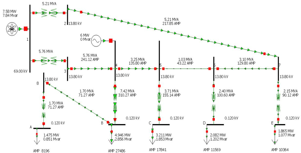
Figure 5: PowerWorld model – Peak Power Demand with the Feeder Battery Connected
