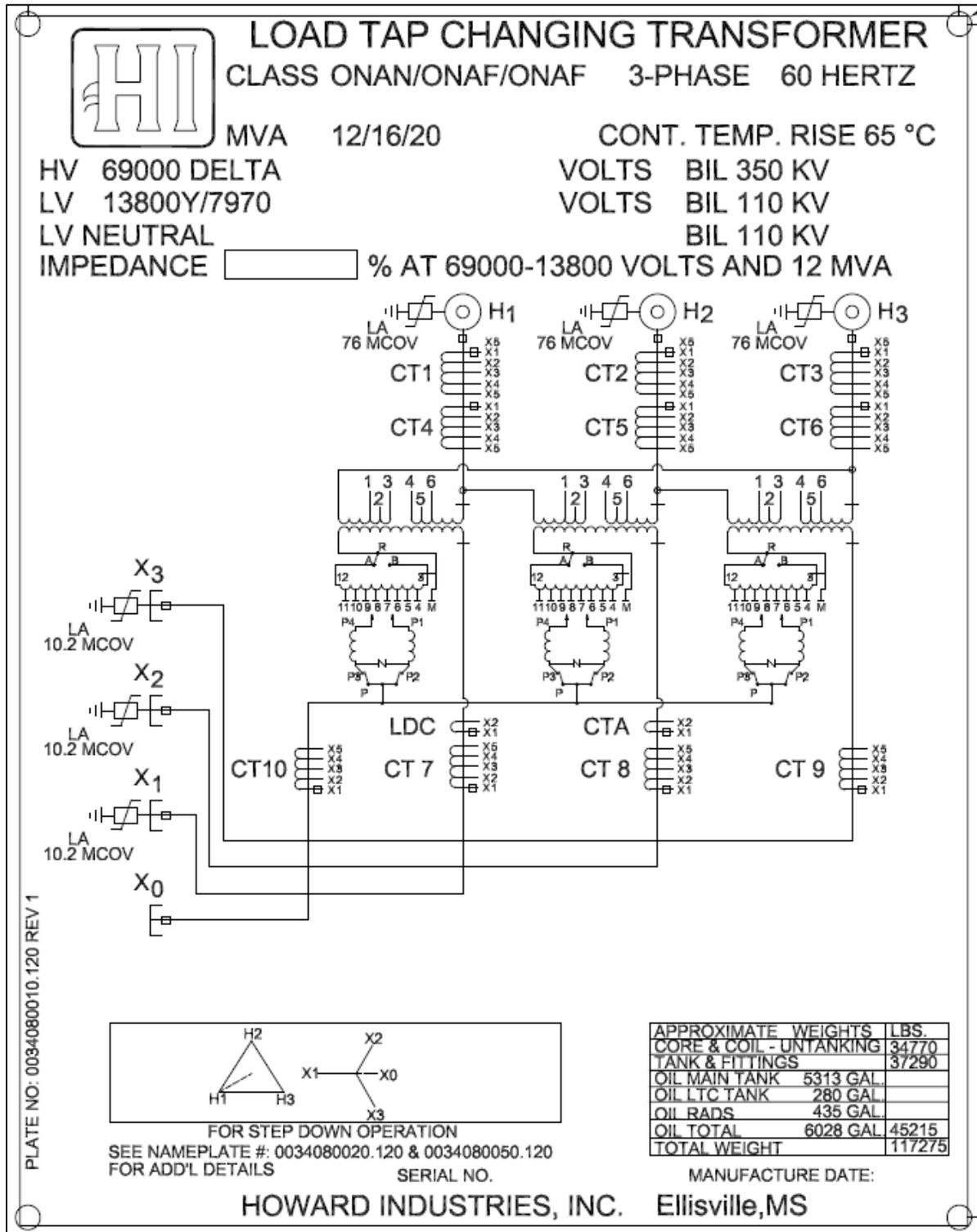
Figure 84: Transformer Specification 1
