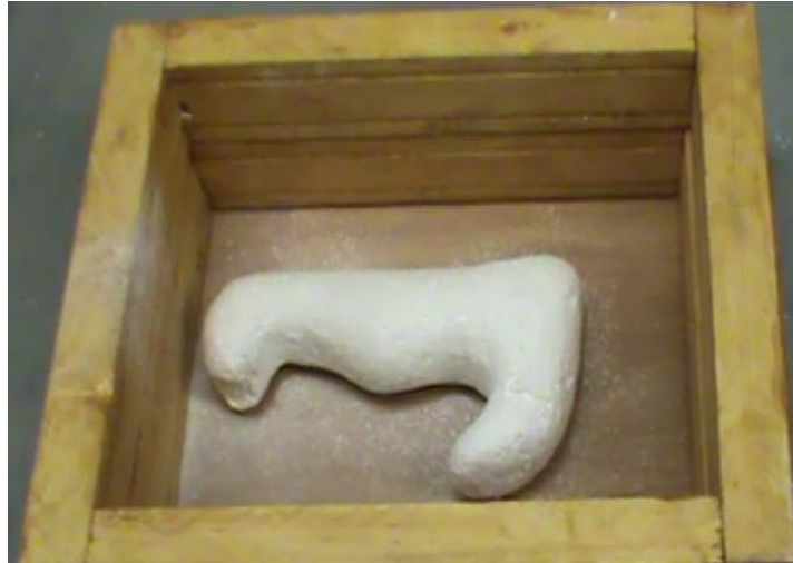
Figure 53: Practice Handle with Parting Dust over it in the Casting Box.
