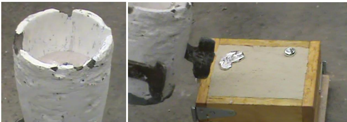
Figure 57: Melted Aluminum and Being Poured into Casting Box.
