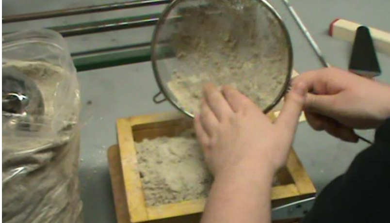
Figure 54: Sand Sifted on Top of Handle and Packed into Casting Box.
