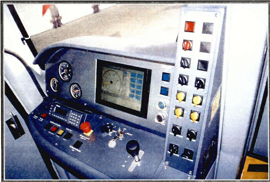
The operator's cab is located at one end of A-car. Control of the train is done from the cab. It is equipped with control console, communication system, adjustable seat, train fault annunciation panel, fire extinguisher, first aid kit and other equipment necessary for operations of the train. Cab can be accessed via cab sliding side door. The cab is air-conditioned. The operator's cab is equipped with evacuation door, which can be in either ramp or sliding mode for controlled evacuation.
