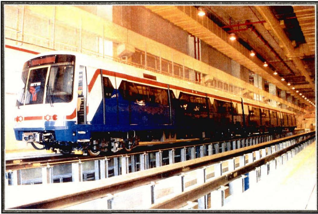
A train is formed by 3- or 6-car coupled together and is capable of running in either direction. The System uses only three-car trains on commencement of operation, and six-car trains will be used when passenger usage of the System rises to beyond the level where the three-car trains can used, a driving car and a trailer car.
