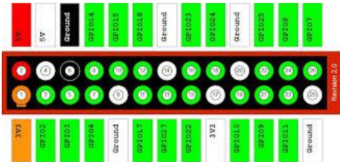
Fig 18 Pins of a Raspberry Pi
