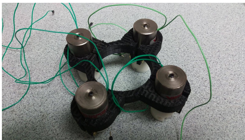
Figure 4.5.2.A: Mounting configuration of Bio-Chem bidirectional pinch valves
