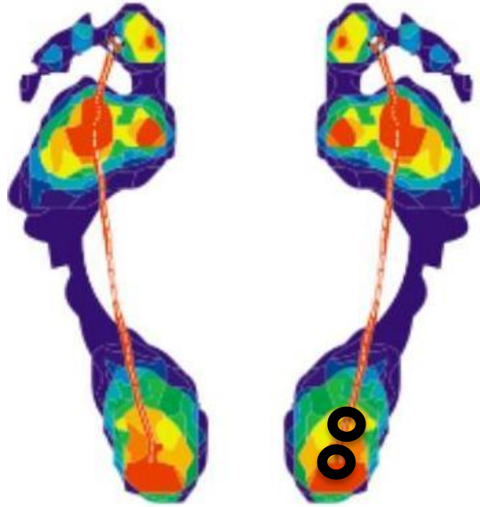
Figure 21: Image of a pair of feet and exactly where the force transducers were placed on the right heel (indicated by the black dots)
