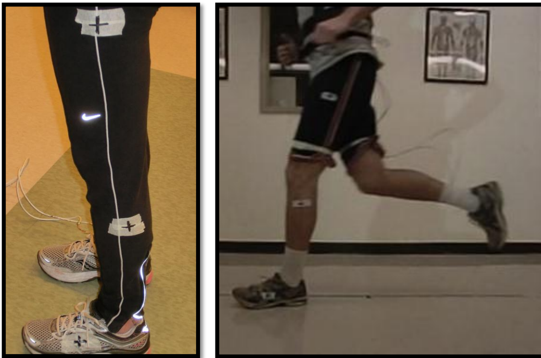
Figure 23: Stationary image of subject with Trackers on the Center of Masses (to the left); Still shot image, tracking of subject while in jogging gait (to the right)
