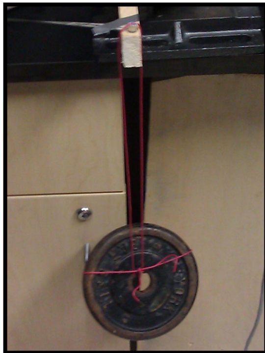
Figure 27: Calibration of Force Transducer using a weight anchored directly on the sensing area of the Force Transducer
