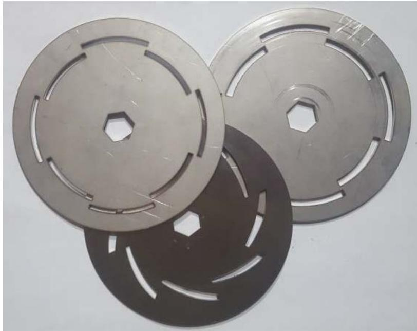
*Figure 16 - Multiple Disks for Testing with the "thin normal" disk top left, "thick normal" disk top right and the thinner tapered disk bottom middle*
