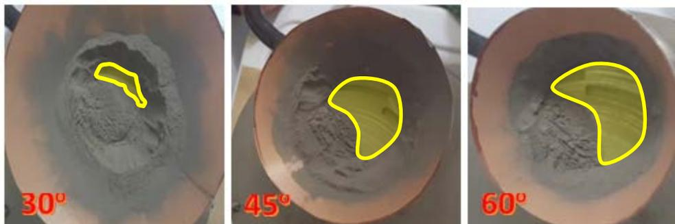
Figure 34 - Pictures taken once all powder was done flowing and the motor was turned off. Notice a large difference between the 30° and 45° but little change between 45° and 60°. The disks are highlighted in yellow to differentiate between remaining powder and the disk..
