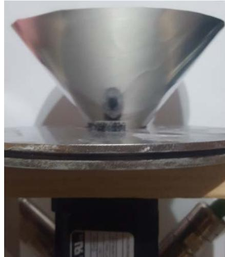
*Figure 36 - Setup of Motor, Disk Assembly and Hopper for Testing*
