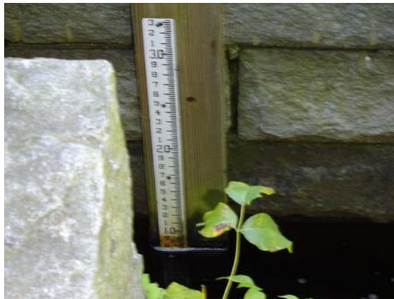
Figure 4.4. Gauging station at site MB1 at the confluence of the Wachusett Reservoir.
