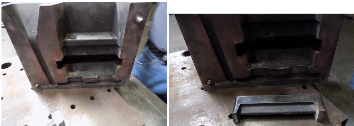
Figure 8: Linamar Mold: Insert Removed from Complex Geometry Side.
