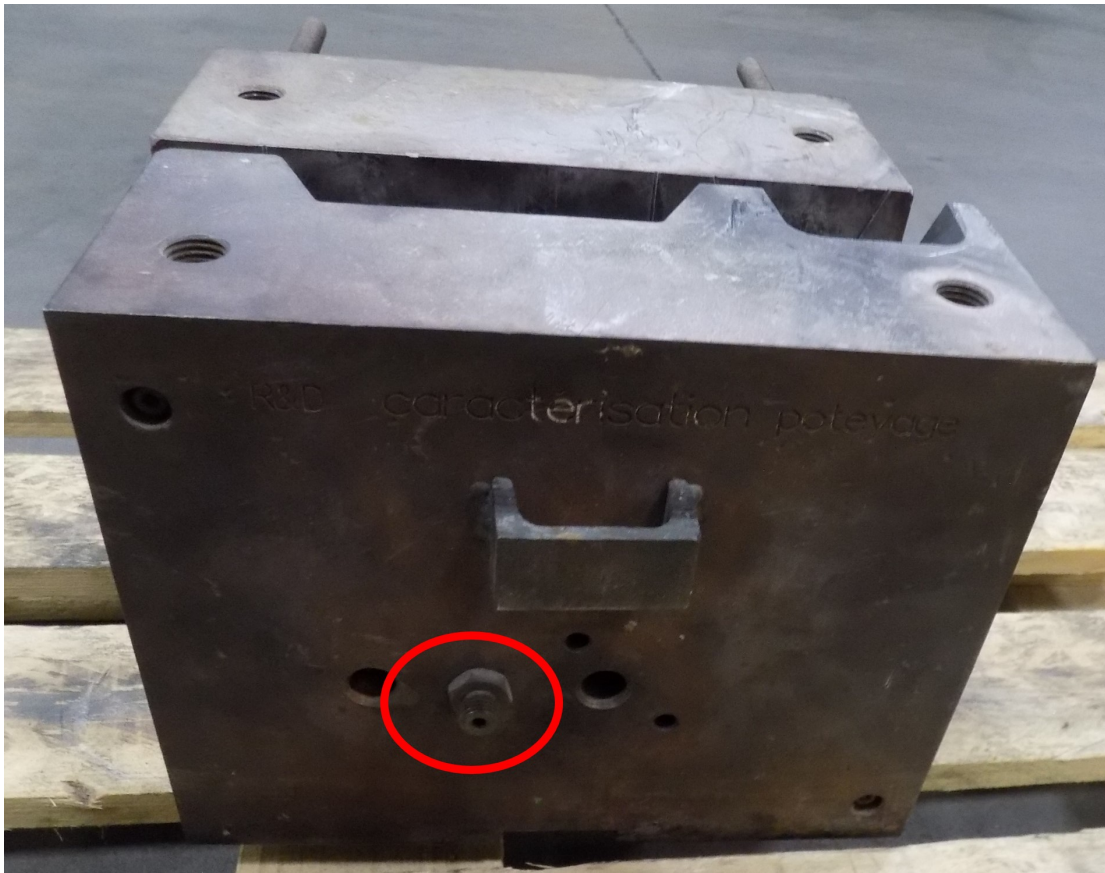
Figure 10: Linamar Mold: (Red) Existing Thermocouple Exit.
