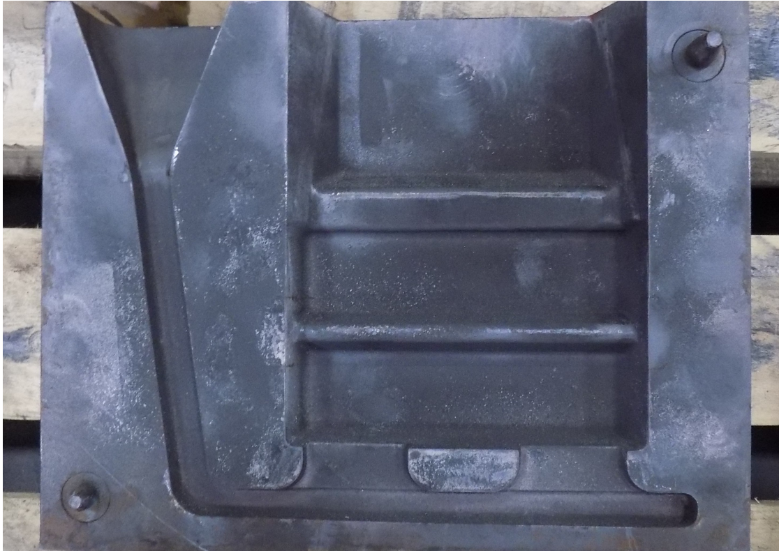
Figure 7: Linamar Mold: Complex Geometry Side.
