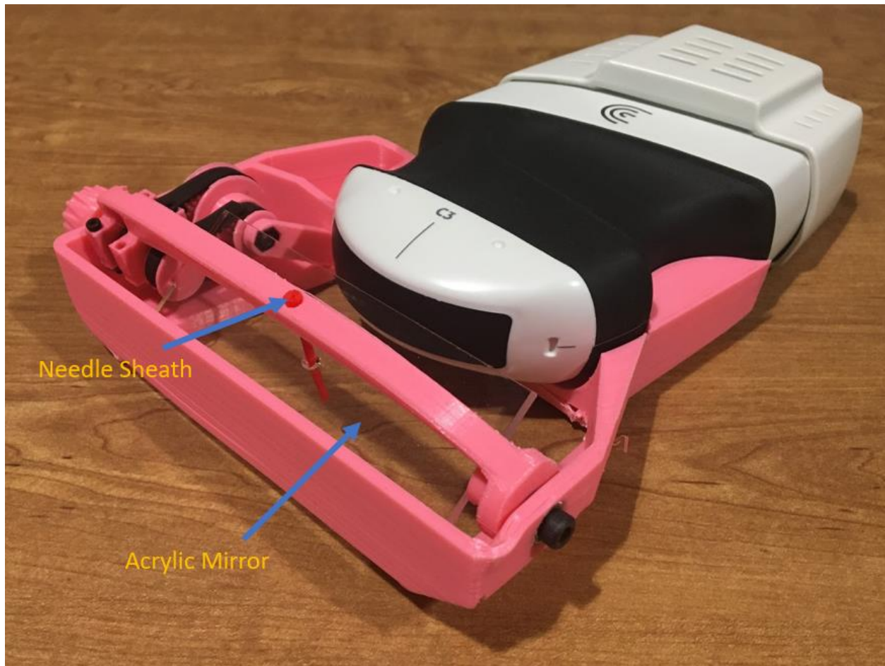
Figure 25: Right Isometric View of Needle-Mirror Mechanism Assembled
