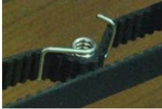
Figure 38: Tensioner Spring Mounted to GT2 belt
