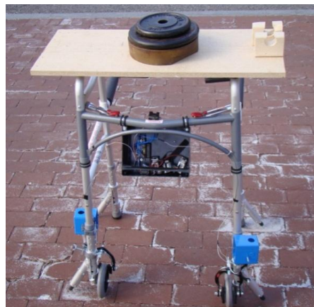
Figure 62: Walker with 38lbf of weight to simulate users' force
