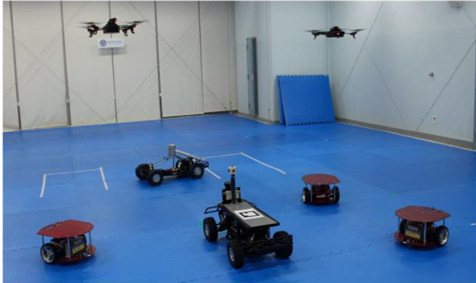
Figure 7.2: An example of a collaborative network consisting of ground and aerial vehicles. Data is relayed from/to the aerial vehicle to/from the ground vehicle to obtain more reliable information and greater accuracy about the vehicles' surroundings [14].
