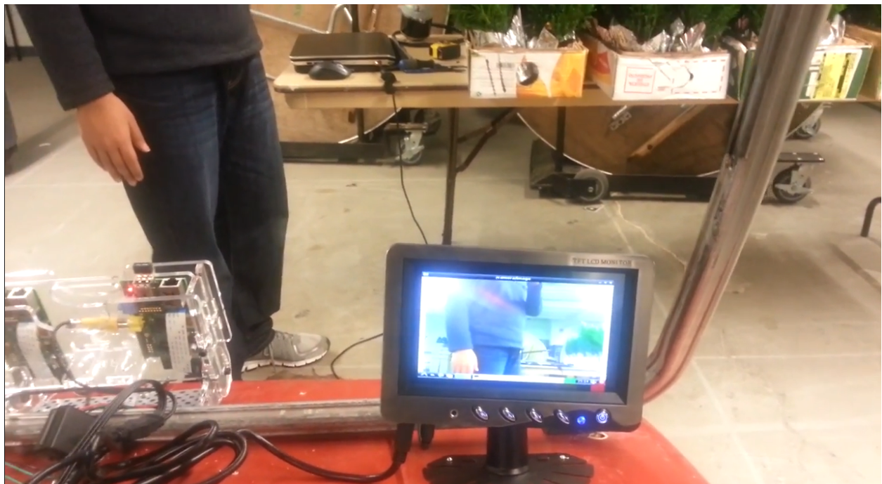
Figure 5.5: The Raspberry Pi Cameras are capturing live data of the surroundings, which is displayed on the Composite Monitor of the IN-DASH system. Images are captured and processed on the Robocart server for object recognition.
