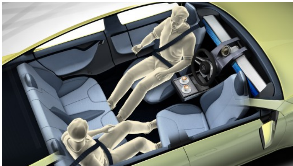
Figure 7.1: Seating Design for Rinspeed's Concept Car: microMAX Urban Vehicle [12]. Rinspeed's microMAX Urban Vehicle is designed with comfort and rotating seating. Front-seat passengers will be able to rotate their seats to face the back-seat passengers while the (autonomous) vehicle drives to the destination [13].
