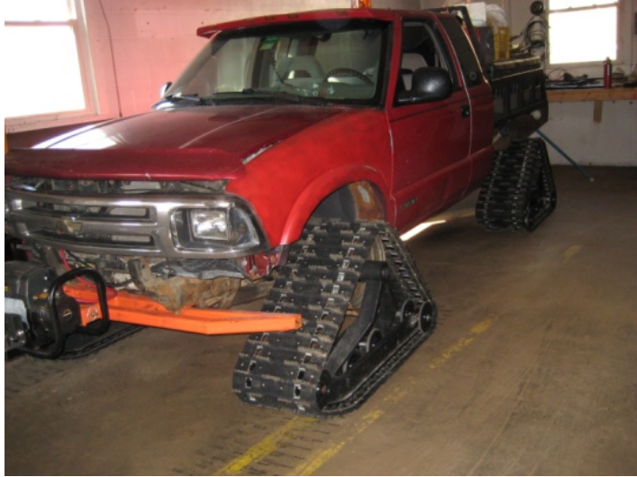
Figure 3: Truck Converted into a Snowmobile Trail Groomer.
