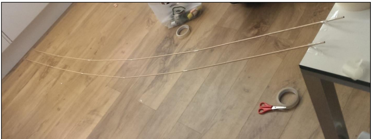
Figure A: Rail sloping from table to floor. Sloping to floor will ensure that rail cars do not derail at the end and break. Notice that the top of the rail is at a slope, not parallel with the table.
