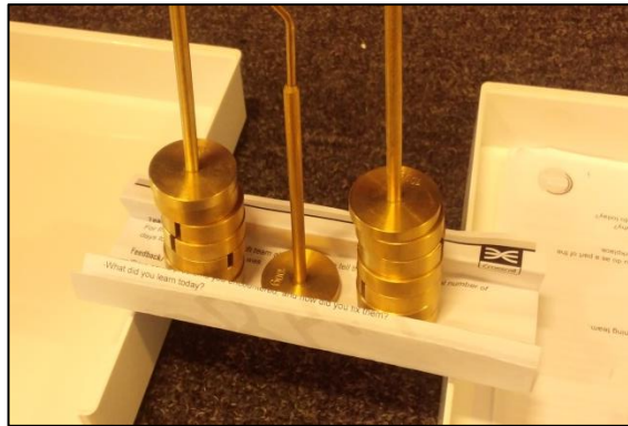
Figure 11: A successful model of the Station Creation bridge made out of two sheets of paper that holds over 1 kilogram of weight
